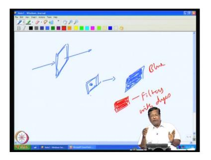
So, basically filters provide a narrow band of radiation. An interference filter, there are difference kinds of filters actually, you can use glass filters, organic dye filters, interference filters and fabry perot etalons. And these glass filters, for example, are simple glass filters like this and they are all colored.
