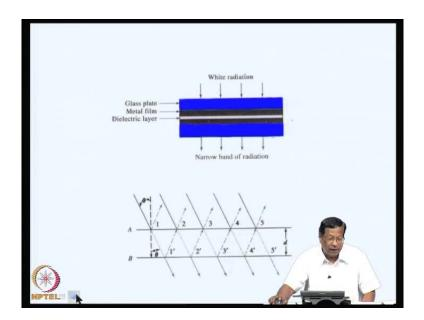
Now, it is essentially the same like what I showed you earlier. These are the glass plates and this is the metal film, this black one. And there is a dielectric layer of calcium fluoride or magnesium fluoride and narrow band of radiation will be coming out of this. And this works on the constructive interference and destructive interference like this, we have discuss these things in the interaction of matter with radiation.
