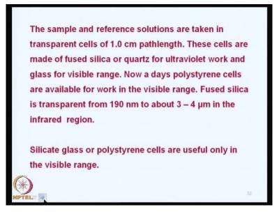
So, the sample and reference solutions are taken in transparent cells of 1 centimeter path length. These cells are made up of fused silica or quartz for ultraviolet work and glass for visible range. Suppose you want to do ultraviolet, work that is work in the range of 180
