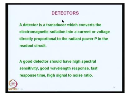
Now, this tell us that bring us to the next part of the instrumentation that is detectors. Now, what is a detector? A detector is basically a transducer which converts the electromagnetic radiation into a current or voltage and it should be directly proportional to the radiant power P in the read out circuit.
