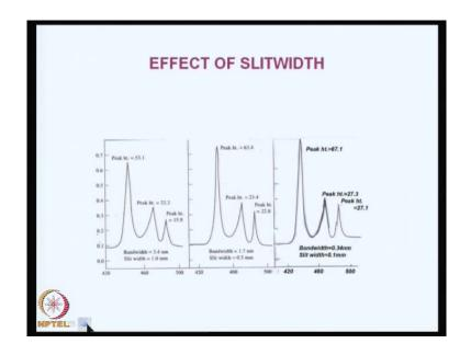
So, you can see the effect of slitwidth here. The first one we have plotted peak height versus wavelength. You can see the peaks are very sharp here. And here the peaks are much better, but peak height you can see as the bandwidth and slit width these 0.5, here it is 1 mm, here it is 0.5 mm, you can see that the peak height here is about 53.1. And as the slit decreases slit width, it goes to 63.4 that is the peak height; that means, the spectrum has become much sharper.
