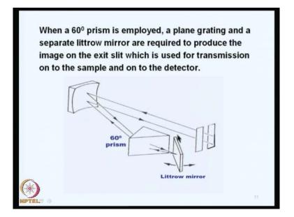
And you can use a prism, 60 degree prism, in carnue mounting. But still here you will see that the littrow mirror has to be on the other site, so the instrument will become slightly bigger, but still you need a littrow mirror to produce the image on the exit slit,
