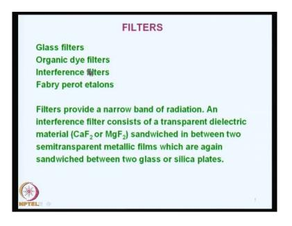
So, we can go for an interference filters. So, what is an interference filter? It consists of a transparent dielectric material for example, calcium fluoride or magnesium fluoride sandwiched between two semi-transparent metallic films, which are again sandwiched between two glass or silica plates.
