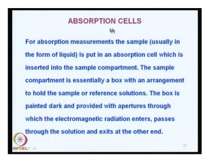
Now, we move on to the other aspect of the spectrophotometric instrumentation, that is the absorption cells. So, absorption measurements, what we do is, we take the sample in the form of liquid and it is put in an absorption cell which is inserted into the sample compartment. What is an absorption cell? An absorption cell is a...
