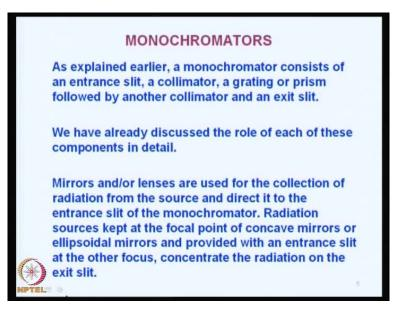
Now, let us discuss about monochromators. Now, what is the monochromators? I have explained to you earlier, a monochromator is an optics system. It consists of an entrance slit, a collimator, a grating or prism followed by another collimator and an exit slit. Instead of grating you can have a filter here, you can have a grating here or you can have a prism there.
