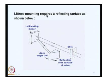
Now, this is a littrow mounting, it requires a reflecting surface like this collimating. So, the slit it will be coming here and then focussed onto the reflecting rear surface of prism and then it passes through it again and then comes back through the entrance slit. This is the arrangement of littrow mounting.
