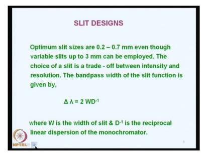
So, the job of the slit is to permit known amount of radiation through a small hole. Basically it is a mechanical operation through which the radiation will be passing through. So, whatever is the size of the slit that will permit radiation to pass through only that, all other radiation will be obstructed. They can be of course, collected in another concave mirror and redirected onto the slit.
