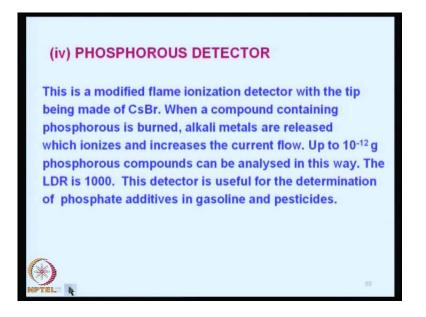
Now, we can discuss a little about phosphorous detector basically a phosphorous detector is a modified flame ionization detector only the difference is that the tip is being made of C C M bromide we just put a small coating of C C M bromide at the tip of the burner.
