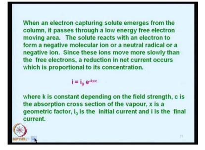
So, this is the electronic capturing solution solute emerges from the column it will pass through a low energy free electron moving area, the solute will react with an electron to form a negative molecular ion. If, the solute reacts with an electron it will acquire negative energy. So, negative charge and then it can form either a negative molecular ion or a neutral radical or a negative ion.
