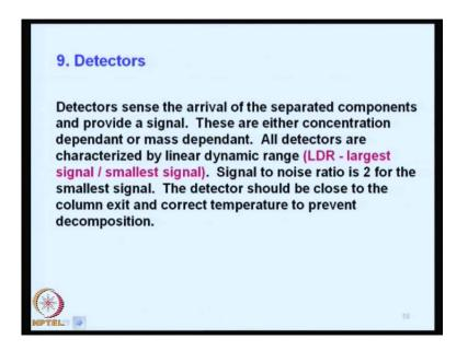
So, in general the detectors sense the arrival of the separated components and provide a signal they these are either concentration dependent or mass dependent; that means, as the concentration of the gas carrier gas changes when the separated component enters the detector, the concentration will change and the concentration will increase to maximum and then it will slowly decrease.
