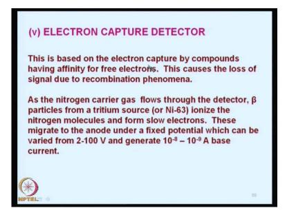
Now, I would like to discuss with you another kind of detector that is known as electron capture detector. This is based on the electron capture by compound having affinity for free electrons. Now, the idea is we have to generate free electrons and these free electrons need to be need to be attracted by the cathode and the during the process it causes the loss of signal due to recombination phenomena.
