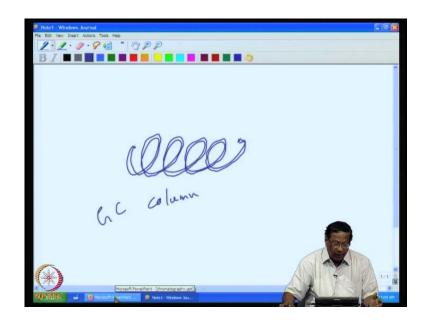
So, this is the gas chromatography column this can be made of the metal as well as it can be made of class, we will see how more about this when we discuss this further. So, what I would like to say at this stage is the gas chromatographic columns are either in u-shape or they are coiled into an open spiral or a flat pan cake type and copper is a useful material for gas chromatography and it is useful up to 250 degree centigrade higher than that is not, so useful.
