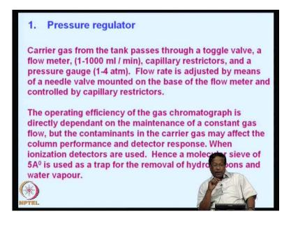
So, let us take a look at the pressure regulator that is the carrier gas system; the carrier gas from the tank passes through a toggle valve and it has a flow meter which will give you about 1 to 1000 milliliters per minute and then it will have capillary restrictors and a pressure gauge of about 1 to 4 atmospheres.
