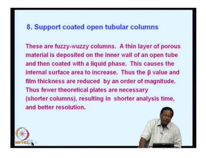
These are known as fuzzy-wuzzy columns. A thin layer of porous material is usually deposited on the inner wall of the open tube and then coated with a liquid phase. This causes the internal surface area also to increase that is a very important concept in fuzzy-wuzzy columns, because of the coating of the liquid inside the capillary the surface area increases.
