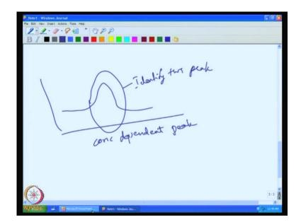
So, this is your basically your carrier gas. So, as the carrier gas as the sample increases, the signal will increase reach its maximum and as it reduces it will come down again to the carrier gas level. So, the job of the detector is to identify this peak; that is, you can identify this peak either of the sample by its specific properties related to concentration or you can use simply the carrier gas.
