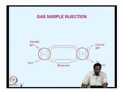
So, whenever you are injecting a sample you have to make sure that the sample does not remain here and in general, that is how? A liquid sample is connected, injected now; this is a gas sample injection through a valve and loop arrangement.
