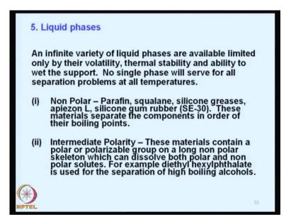
So, the liquid phases are usually can have a number of liquid phases they are readily available and there use is only limited by their volatility, thermal stability and ability to get the support it is a very important parameter, the support must also be wetted by the liquid to form a thin film membrane over the material.
