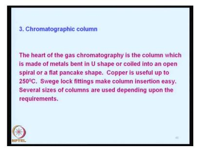
So the next part, what we want to discuss? Is about the chromatographic column as I told you, the chromatographic column is basically the heart of the gas chromatography it is the column which is made of metals; it is a metal tube basically it is bent in U shape or coiled into an open tube, why do we need this coiling? Is because, it will occupy less space. So, this is how a column will look.
