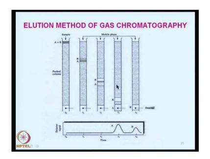
Now elution method of gas chromatography is something like this that is I have A column here and the sample is here A plus B I have a packed column and in this column you can see this small small particles on which liquid is coated, but that is not visible and the sample is introduced from the top and then I have the packet column gases passing through and then this plug will start moving at its own speed and depending upon the
