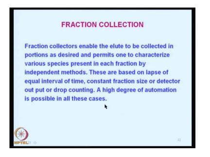
Now, I am talking about fraction collection that is a fraction collectors what are their jobs their job is to enable the elute to be collected in portions as desired and permits one to characterized various species present in each fraction by independent methods.
