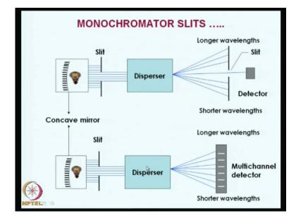
To tell you very frankly, we are talking about slits. And, there is no mechanical interaction except that these slits allow the radiation from one end up to the other end; that is, it will allow the radiation to pass through with a fixed aperture. Usually, in all spectrophotometers, etcetera, you need two slits: one is the entrance slit and another is the exit slit.
