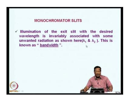
Illumination of the exit slit with the desired wavelength is invariably associated with some unwanted radiation as shown here lambda 1 and lambda 2, which I did not show it there. This is known as bandwidth.
