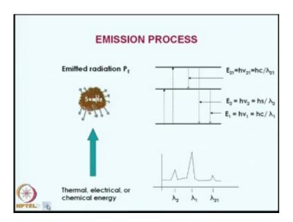
For example, you can see here. This is basically an emission process. Here I have the sample; I am giving stimuli here. It may be thermal electrical or chemical energy. And, here the energy levels are there: E 1 is equal to h nu 1 or h c by lambda 1; E 2 should be h nu 2 or h c by lambda 2; E 2 1 should be h nu 2 1 or h c by lambda 2 1. So, these are the different wavelengths that are coming out of the system. So, this is one type of stimuli.
