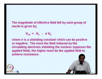
So, you would get different kinds of spectra defined by the shielding constant given by, H 0 minus sigma H 0; this we have already discussed. But, what is more important is? The more the field is induced by the circulating electrons shielding the nucleus, the higher must be the applied field to achieve resonance. The field is more; field applied field also should be more to obtain the resonance.
