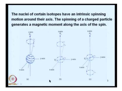
That is this, here I have the applied field here and the moment the magnetic frequency is matched by the applied field, the spin will be changed in the opposite direction like this; first it was on the top, now it is on the at the bottom. So, this is known as the frequency at which this happens is known as lamer frequency. (Refer Slide Time: 13:41)
