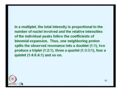
So, in a multi plate, the total intensity also varies according to the proportional to the number of nuclei involved and the individual peaks follow the coefficients of binomial expansion. For example, one neighboring proton splits the observed resonance into a double and two will produce a triplet of 1 is to 2 is to 1, ratio three would be a quartet with 1 is to 3 is to 3 is to 1 and four would be a quintet with 1 is to 4 is to 6 is to 4 is to 1 etcetera.
