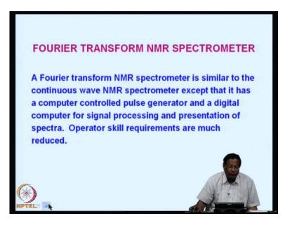
So, FTNMR spectrometer is similar to the continuous wave NMR except that it has a computer controlled pulse generator and a digital computer for signal processing and presentation of the spectra. So, operator skill requirements are much reduced in FTNMR.
