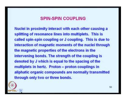
Now, let us discuss about the spin-spin coupling. Nuclei in proximity with each other causing a splitting of resonance lines into multiples. So, this I have shown you a figure of
