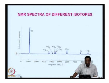
So, like that one can calculate, what are the different numbers involved? this is the NMR spectrum of different isotopes, here you can see 1 H assuming that this is around 100, we can see that intensities of the peaks or instrument response is for boron, copper and then sodium, etcetera they are all very small compare to protons and silicon is slightly better 2 H is very less, and this is the x axis is the magnetic field.
