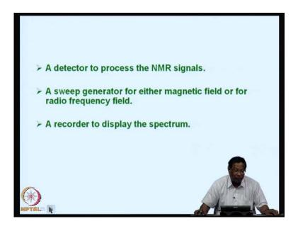
A then you need a sample probe containing coils for coupling the sample with the r f field. That is also important; that means, the sample also must be having some short of a coil, which can couple with the applied r f field. And a detector you need to process the
