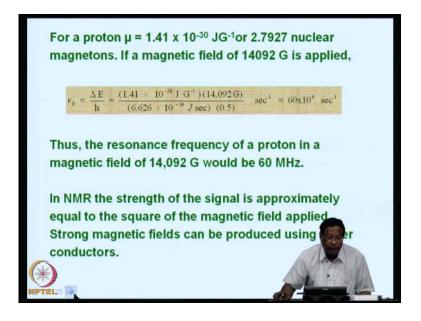
So, for a proton we have the momentum corresponding to 1.41 into 10 raise to minus 30 joules per gauss inverse or 2.7927 nuclear magnetrons. So, if a magnetic field of 14,092 gauss is applied, then we can we can calculate the frequency corresponding to the change and you would end up with 60 into 10 raise to 6 seconds inverse.
