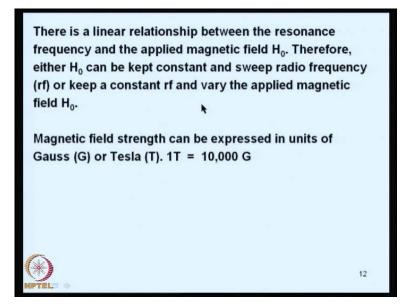
So, there is a linear relationship between the resonance frequencies of the applied magnetic field H 0. Therefore, we can either keep H 0 as constant and sweep the radio frequency or keep the radio frequency constant and vary the applied magnetic field H 0. Therefore, this gives us two ways of running a and NMR spectrometry. So, magnetic field strength usually is expressed in terms of gauss or tesla; and one tesla corresponds to about 10000 gauss.
