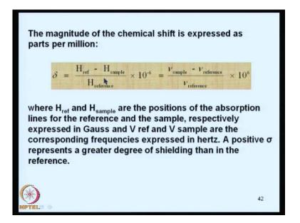
So, the magnitude of the chemical shift is expressed as simple equation like this; that is delta is equal to H reference minus H sample by H reference multiplied by 10 raise to minus 6 that is for the applied field; and which can be converted which is almost equal into v reference v sample and multiplied by 10 raise to 6. So, positive delta shift represents greater degree of shielding than the reference.
