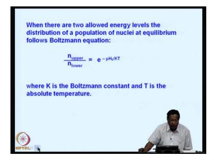
So, when there are two allowed energy levels the distribution of a population of nuclei at equilibrium follows the Boltzmann distribution, what is Boltzmann distribution? It is this part of e to the power minus mu H 0 upon K T. where, K is the Boltzmann constant and T is the absolute temperature. So, the distribution in the upper energy state to compare to the lower energy state; that is the ratio is governed by the Boltzmann equation.
