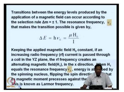
So, the transitions between the energy levels produced by the application of the magnetic field can occur; according to the selection rule, delta m should be changing only by whole numbers; that is plus or minus 1.
