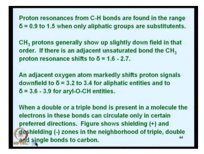
So, here you can see this is the triple bond, and this is the double bond; this shielding effect is like this and the this is minus, this is plus and this is plus and this is for aromatic compounds induced magnetic fields have got to be above the basic ring structure and below the basic ring structure. So, the electrons are got to be moving around it like this similarly on the other side also.
