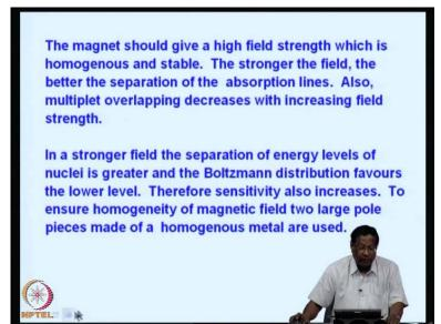
So, this is how? You would see a NMR spectrum and the magnet should give a very high field strength which is homogenous and stable. The stronger the magnetic field the better is the separation of the absorption lines. Also, multiple overlapping decreases with increasing field strength.
