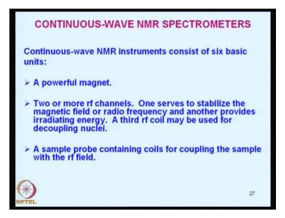
So, continuous-wave NMR spectra meters consist of six basic units: one is you need A powerful magnet and you need two or more r f channels. I had explained to you this earlier, one serves to stabilize the magnetic field or radio frequency and another provides irradiating energy. A third r f coil may be used for decoupling the nuclei.
