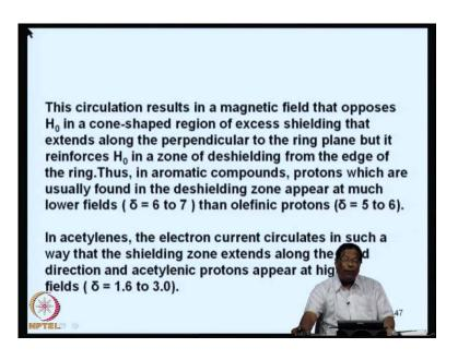
So, the circulation results in a magnetic field that opposes the applied magnetic field H 0 in a cone-shaped region of excess shielding that extends along the particular that extends of along the perpendicular to the ring plane, but reinforces H 0 in a zone of deshielding from the age of the ring. Thus, in aromatic compound protons which are usually found in the deshielding zone appear at much lower fields approximately delta shift should be between 6 and 7.
