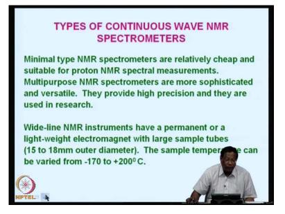
So, minimal types of NMR; minimal type of NMR spectrometers are relatively cheap and suitable for proton NMR measurements. Multipurpose NMR spectrometers are more sophisticated line and they are versatile. They provide high precision and they are used in research. Wide-line NMR spectra instruments spectrometers have a permanent or a lightweight electromagnet with large sample tubes. And the sample temperature can be varied from minus 170 to 200 degree centigrade.
