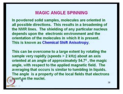
So, in powdered solid samples, molecules are oriented in all possible directions. This results in broadening of the NMRS lines. The shielding of any particular nucleus depends upon the electronic environment and the orientation of the molecules in which it is present. This is known as Chemical Shift Anisotropy.
