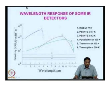
Now, the wavelength response you can make thermocouples of different materials, for example, you can make this one figure, the first one is indium antimony, this is the response at 77 Kelvin. So, this scale is detectivity is 10 raised to 8 to 10 raised to 11; this starts somewhere around 10 raised to 10 then falls off around 5 micro meters.
