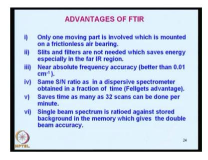
Now, you can see that there are there are only few moving parts, in the, in the, in using f t i r, there is actually one moving part in is involved, that is the moving mirror, which is
