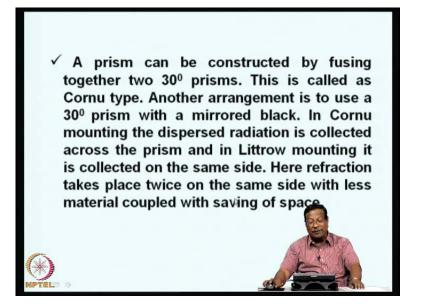
A prism this is called Cornu. And, mirrored black, etcetera – this I have already referred to you. Here the refraction takes place twice on the same side with less material coupled with the saving of space.
