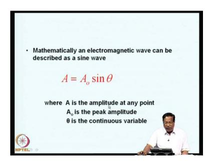
Such a plane-polarized wave is represented mathematically. So, mathematically, an electromagnetic wave can be described as a sine wave something like this – A is equal to A 0 into sine theta; where, A is the amplitude at any point; A 0 is the peak amplitude; and, theta is the continuous variable.
