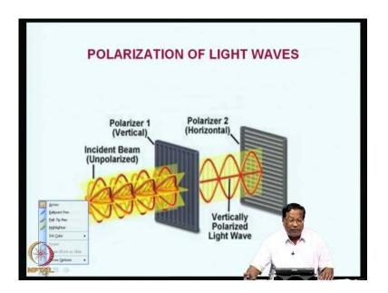
Basically, what you see when a light beam is passing around, you would see that the electronic vectors are there, magnetic vectors are there. A beam of light passing through a media – if you view it from the receivers end, that is, if the light is coming towards the observer, you would see a number of beams, a number of parts that is electrical and magnetic part bundled together in not so systematic manner. But, it is a big bundle
