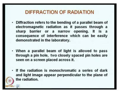
Diffraction refers to the bending of a parallel beam of electromagnetic radiation as it passes through a sharp barrier or a narrow opening. It is a consequence of interference, which can be easily demonstrated in the laboratory. When a parallel beam of light is allowed to pass through a pinhole, two closely spaced pinholes are seen on a screen placed across it.
