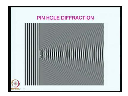
If the radiation is monochromatic, what you would see is a series of dark and light images appearing perpendicular to the plane of radiation like this. So, here we have a radiation going along and we have a small this thing - a pinhole; and, the radiation that are coming out on this side, where we place a screen on this side, you would see a sharp image of black and white, black and white, black and white. So, this phenomenon is diffraction.
