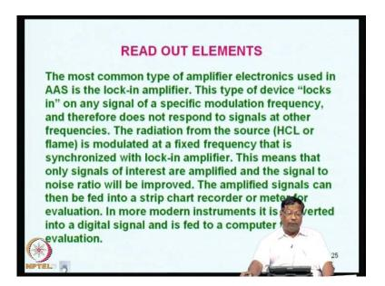
So, but just for the sake of brevity and putting most of the words into this slide to make it clear to you. So, the if you proceed to the read out elements again we have discussed that lock in amplifiers have got very important function to measure the response only at a particular frequency. And this frequency is locked; that means, the all other frequency would be rejected from the strip chart recorder.
