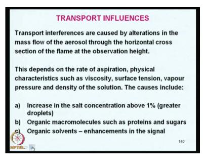
because the monochromator cannot handled this. Sometimes I have also told you that transporting infer influence. These transport interferences are caused by the alterations in the mass flow of the aerosol through the horizontal cross section of the flame, at the absorption height. This depends on the rate of aspiration physical characteristic such as viscosity, surface tension, vapor pressure, and density of the solution etcetera.
