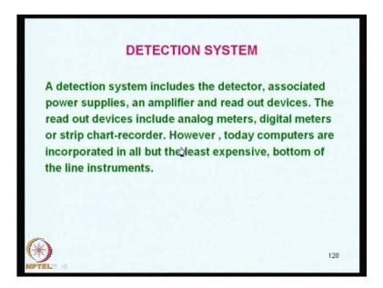
and read out devices. The read out devices include analog meters digital meters or a strip chart recorder; however, today computers are incorporated in all, but the least expensive bottom of the line instruments the while continuing the our discussion on the detectors in the last class (Refer Slide Time: 00:52)
