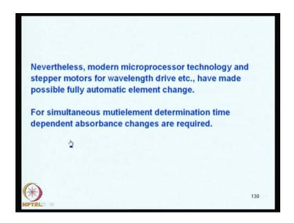
and uses stepper motors for wave length and setting slide etcetera. They have they are now they are completely made automatic and for simultaneous multi element determination time dependent absorption changes are also required. For example, if you want to determine number of elements in the same sample, some it is possible to run through a sample number one to number 10.
