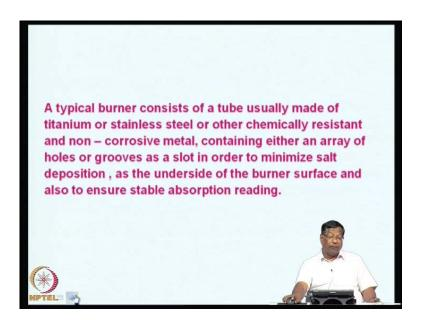
So, a typical burner usually consists of a titanium base or a stainless steel base. So, other there are other chemically resistant and a non corrosive metals also have been used, but mostly titanium as well as, stainless steel burner seems to be of use. They contain either and array of holes or grooves as I slot in order to minimize salt deposition has the underside of the burner surface and also to ensure stable absorption. (Refer Slide Time: 03:36)
