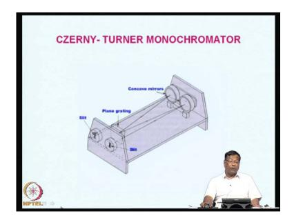
And if we go to Czerny Turner mountain it is a again fairly simple arrangement. We have silts here one silt here, one silt here and a plane grating is placed in front of them and conquered mirrors are there. So, that radiation coming through this silt will go on to the conquer mirror reach the grating and then again go back to another mirror and it comes back through the exit silt. Very simple arrangement both these arrangements are
