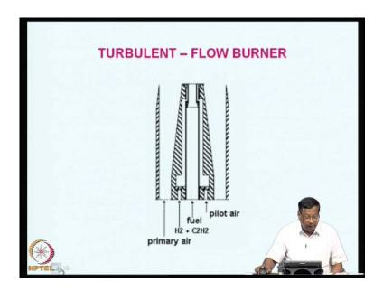
So, a typical burner we have to make it like this, and the actual design of the burner is like this, here we are introducing primary air and then there will be hydrogen possibility for introduction of hydrogen and acetylene and fuel also would enter like this. And pilot air, if we are using air as an oxidizer we are going to mix all of this is a material, which is at the edge is made of titanium here as well as outside.
