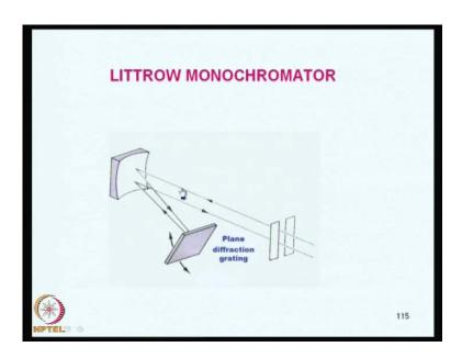
And this is mono Littrow monochromator we have an entrance exit silt here and this is Littrow mounting.
