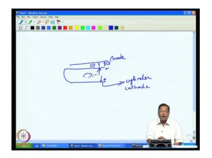
what do you mean is the ions, this is your hollow cathode lamp and then there is argon gas filled here in all the spaces and the positive ions will strike the cathode and the negative ions will strike the anode. This is anode negative ions and positive ions will go and hit the cylinder, this is in the form of a cylinder and that is cathode. This is the basic process in which the ions will come and bombard the cathode.
