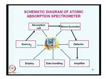
Now, let us take a look at the architecture of atomic absorption spectrometer, now my next slide shows you the basic component of the atomic absorption and like all other instruments, here you need a source that is here. And then you need an absorption cell, where you can produce the atoms in the ground state and then what happens from the source radiation is passed through the absorption cell and then you need a monochromator to separate unwanted radiations.
