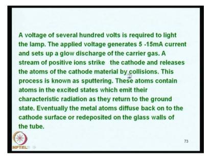
Whenever we start operating, the hollow cathode lamp, so you take a hollow cathode lamp fill it will neon or argon set up a glow discharge and positive ions will strike the cathode and releases the atoms of the cathode material by collision.
