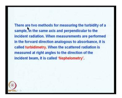
Now, under these conditions, there are two methods for measuring the turbidity of a sample. One is in the same axis and another is perpendicular to the incident radiation. Now, I will show you very simple arrangement.
