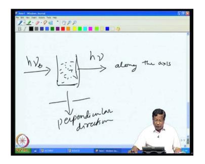
How you can measure the absorbance? Here is your sample, here is your incoming radiation and then, you can choose to measure this is h miu 0, this is h miu, this is 0 and this is your sample holder. This contains the sample and this contains the substance. Now, you can measure along this direction or you can measure along this direction. This is perpendicular, this is perpendicular and this is along the axis. So, the one is called Nephelometry and another is called Turbidimetry.
