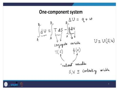
We have already established that the change in the internal energy is given by the heat added and the work done on the system and in the differential form we can write this as-
