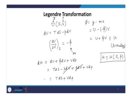
So just like what we did earlier was we had y as a function of x and I defined a slope and I defined an intercept  $\Phi$  but in reality what you have is a multivariable function. So you have U as a function of both S and V that means I need to define two slopes in terms of two variables that we have in the problem x1 and x2. So I can extend this idea and what we then have and you can derive it is I can define the intercept as-
