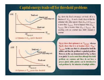
Now this is the operating cost which changes from this point to this point and remains constants to this to this and; obviously, this is the t threshold; up to T threshold the utility demand remains constant, whether it is a hot utility demand or a cold utility demand. So, the operating cost remains constant up to the T threshold and then it increases, but the fixed cost decreases when I increase the delta T minimum, I am providing more delta T;
