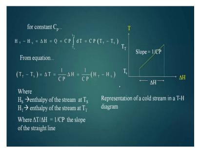
Now, for constant c p we see that this will c p will come out of the integration and we will see this relationship c p equal to t t minus t s and this forms the equation after knowing how to place a cold stream in a t h diagram the second job is to integrate it before we start integration let us see the property of this t h diagram that what it allows and what it does not allow.
