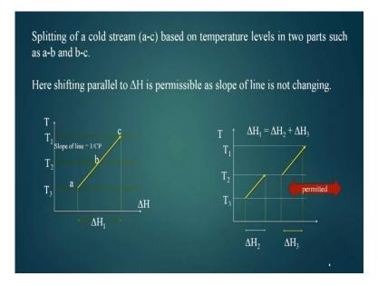
Let us see a second property that whether the cold stream can be splitted or not now this shows a cold stream which is operating in the temperature interval t one and t three where t three is the supply temperature and t one is the target temperature and it slope is one by c p.
