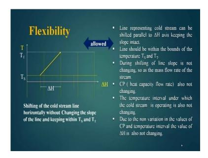
Now, in this figure let us see there is a cold stream which start from supply temperature t s to t t was slope is constant and it requires delta h amount of enthalpy to heat it from t s
