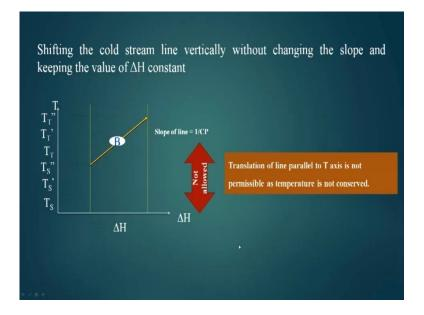
Let us see in the t h diagram if a cold stream is shifted vertically then what happens for this purpose we are showing a cold stream which supply temperature is t s and target temperature is t t. Now it slopes is one by c p and while translating it vertically upward I am not changing c p value; that means, I am not changing.
