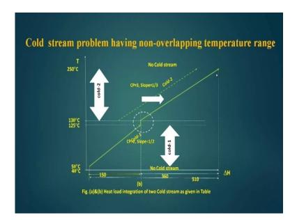
Now, this shows the temperature levels of two cold streams the first cold stream temperature level is from 50 to 125, and for the second cold stream it is 130 to 250 and there is gap here 125 to 130 were is where no cold stream is present now if I want to join
