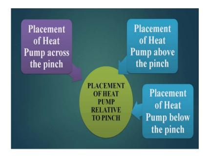
Now let us take the placement of heat pump across the pinch. So, when I talk about the placement of the heat pump, we saw this pinch then it can be above the pinch, it can the below the pinch or it can be across the pinch. So, there are three places for placement, and we have to check all these three places, and see where the placement is beneficial and where should not place the heat pump.
