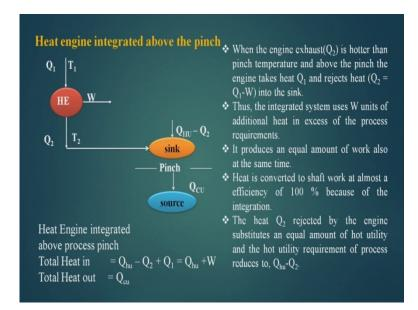
Now this is a process, this is the heat engine. Now if I am placing like this, I am taking Q 1 and rejecting Q 2 to this. If I do so, my hot utility decreases by Q HU minus Q 2. So, heat engine integrated with the above pinch, my total heat in is Q HU minus Q 2 plus Q
