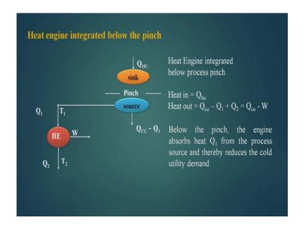
Now if I am integrating it below the pinch, the heat engine integrated below the pinch, I am taking Q 1 heat from below the pinch and rejecting it into the cold water. So, the demand of the cold utility for the process is Q CU minus Q 1, so this is Q CU minus W. Below the pinch the engine absorbs Q 1 from the process source and thereby reduces the cold utility demand.
