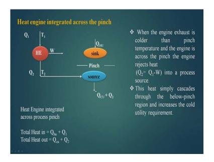
Now we see across the pinch. Heat engine integrated across the pinch. When the engine exhaust is colder than the pinch temperature and the engine is across the pinch the engine rejects Q 2 amount of it into the process source. So, it is rejecting Q 2 amount of heat into this process source which is below pinch. This heat simply cascades through the below-pinch region and increases the cold utility requirement, so it has increases the cold utility requirement.
