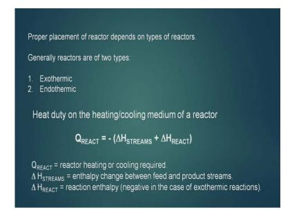
Now the proper placement of reactor depends upon type of reactors. Generally reactor are of two types – exothermic, endothermic. Heat duty on the heating cooling medium of a reactor can be retain like this Q reactor is equal to minus delta H streams plus delta H reactants. And Q react is there reactor heating or cooling requirement, delta H streams is enthalpy change between the feed and product streams, and delta H react is reaction enthalpy negative in the case of exothermic reactions.
