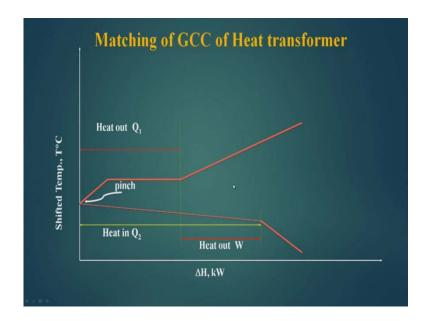
This is for heat transformer this is the amount of heat, which is available a part of heat this much is upgraded and this is a downgraded. So, we get less heat here in a heat transformer which is a upgraded heat.
