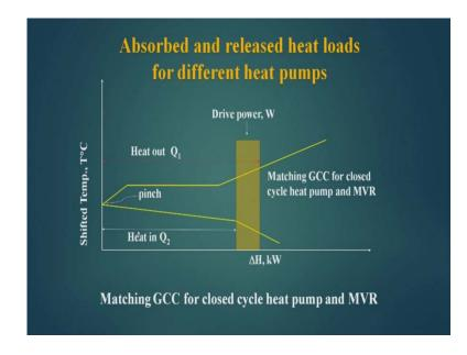
Now, if you see that absorbed and released heat loads of different heat pumps, if I am using a closed cycle heat pump. So, this is the amount of Q 2 it picks up the distance between this and this is the amount of Q 2 its picks up, and deliver is from here to here; that means, this band is for driving power. So, this much amount it will pick up and this much amount it will deliver.
