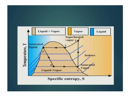
This is the entropy-temperature, entropy diagram. This is the compression part then superheating then condensing then expansion then vaporization takes place.
