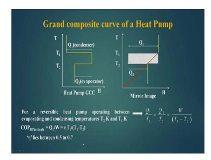
Now let us see the a heat pump, now the if I plot the heat pump this will look like this this is the evaporator and this is the condenser because the less heat, that is Q 2 will be taken from the evaporator and more evaporator will producing the condenser. So, this look like this. So, if I get a mirror image of this. So, this will look like this now for reversible heat pumps operating between evaporating and condensing temperatures T 2
