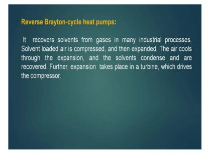
Reverse Brayton-cycle heat pumps it recovers solvent this pump recovers solvents from gases in many industrial processes solvent loaded air is compressed, and then expanded the air cools through the expansion, and the solvent condense and are recovered further expansion takes place in a turbine which drives the compression.
