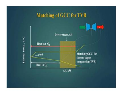
Now, for thermal vapour compression units this much amount it picks up, and this much amount it delivers and it is the driver steam systems delta H. So, it adds up to this Q 2
