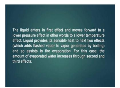
So, it is again within the steam and cold water temperature levels, this falls within this temperature levels. The liquid enters in the first effect and moves forward to a lower pressure effect. In other words to a lower temperature effect, liquid provides its sensible heat to the next two effects, which adds flashed vapor to vapor generated by boiling, and so assist in the evaporation. For this case the amount of evaporated water increases through second and third effects.
