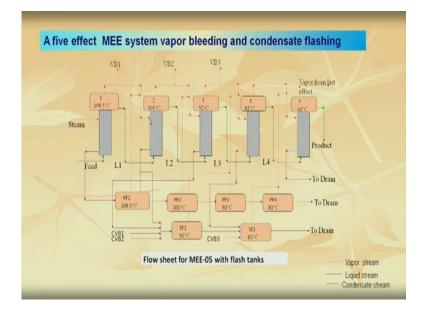
Now, let us take see two more things in multiple effect evaporator, one is called vapor bleeding and another is called condensate flashing, what does it mean? Now see this is a five effective evaporator system with vapor bleeding as well as condensate flashing. Now, this here I mean the first effect I am feeding steam and the condensate of the first effect goes to a flasher, here its pressure is decreased and flash steam is generated and that is flash steam joins the vapor to the second effect.
