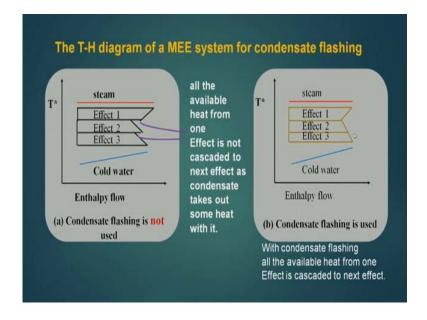
Now, this shows the condensate flashing is not used, if I am not using the condensate flashing this may look likes something like this because this much of heat, goes away with the condensate. So, my a MEE diagram will look something like this, but if I am using condensate flashing, this will look like this because I am to some extent regaining that heat which is being lost.
