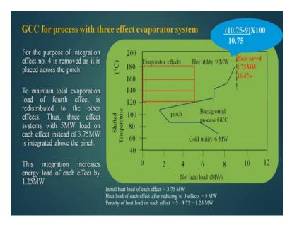
But I have increased the load of each evaporator, so this can be shifted invert. So, the lower from 3.75 megawatt I have increase it to 5 megawatt so 3.75 into 4 and 5 into 3 are same. Now, the hot utility requirement is 9 megawatt. So decrease in hot utility requirement is now 16.3 so by converting a 4 effect evaporator to a 3 effect evaporator. And while doing so increasing the head load of each evaporator to 5 megawatt, will do a saving of about 16.3 percent.
