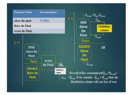
Now, the distillation column can be integrated above the pinch or it can be integrated across the pinch. When it is integrated across the pinch it takes Q reboiler from above the pinch area and r jets Q condenser in the below the pinch area when it does. So, we call it that it is been integrated across the pinch or it can be integrated below the pinch. In the below the pinch it is taking Q reboiler from below the pinch and injecting Q condenser below the pinch.
