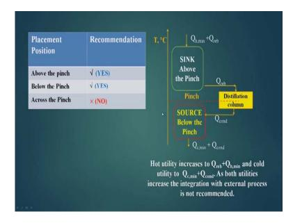
So, my hot utility consumption increases by reboiler, so Q h minimum plus Q reboiler. Because, this area the system is deficient of heat and that is why I am taking heat from outside. So, if I take heat further from here, so this outside heat has to increase to satisfy this. So, my hot utility requirement has increased from Q H minimum to Q plus reboiler
