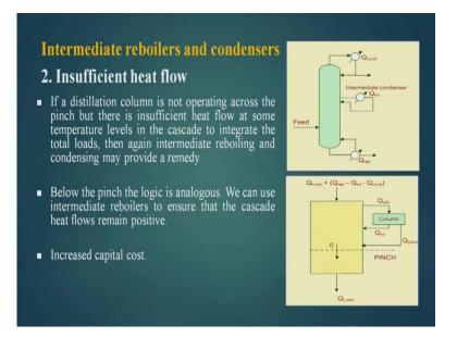
Now, if there is in sufficient heat flow that we have seen that insufficient heat flow like here I will show the picture. Here the condition is that Q 3 should be more than Q condenser. Here the Q 2 should be more than Q condenser here when I am integrating above the pinch.
