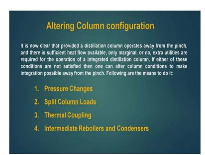
Now, it is now clear that provided a distillation column operates away from the pinch and there is sufficient heat flow available only marginal, or no, extra utilities are required for the operation of a integrated distillation column. This way have seen very clearly that for the upper pinch area if it is integrated it almost runs free of cost or with marginal increase in the utility.
