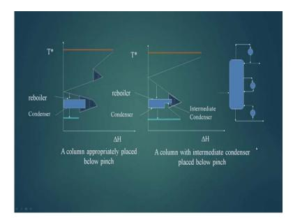
Now, let us see how this will be integrated below the pinch this is physical aspect, let see then will consider the placement across the pinch. So, when I am putting up a distillation column below the pinch it will look like this. So, the heat, which is available from here to here by the process stream will be given to reboiler and the heat, which is available from this to this, is also given to the reboiler.
