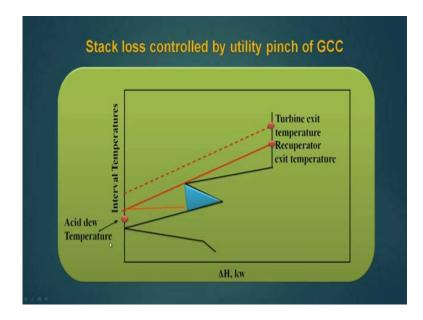
Now, there is utility pinch here what we see that this area where there is a utility pinch controls that the temperature, this is acid dew point and I should come to this acid dew point. That means, the this line should cross this, if it cross then the real job has been done otherwise there is a loss, I am not able to sue this much of heat and why this is not able to cross this acid dew point because there is a utility pinch here. So, as the maximum heat has to be tangent to this point.
