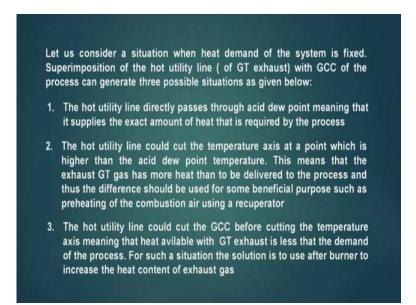
Let us consider a situation when heat demand of the system is fixed. Superimposition of the hot utility line that is G T exhaust with G C C of the process can generate, three possible situations as given below. The first situation is the hot utility line directly passes through the acid dew point meaning that it supplies the exact amount of heat, that is required by the process. This is very ideal situation and we will always welcome this.
