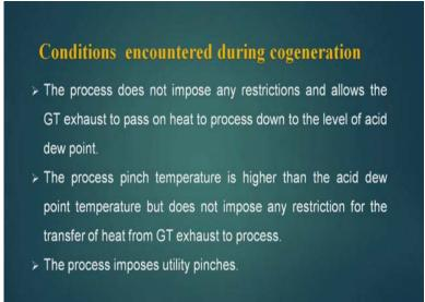
So by calculating this expressions, we can find out this C total cost and this will be automatically annualized cost or the stack. Now, the conditions encountered during cogeneration let us analyze this. The first point is the process does not impose any restriction and allow the G T exhaust to pass on heat to process down to the level of acid dew point. If it is not imposing any restriction this is say free problem and easier to tackle.
