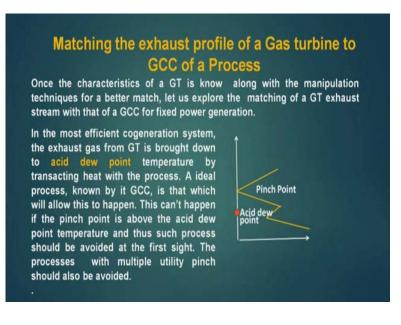
Once the characteristic of G T is known along with the manipulation techniques which we have seen using of after burners a better match can be done. So, let us explore the matching of G T exhaust stream with that of G C C for a fixed power generation. Now, let us see, when a cogeneration system in which we are producing power, and the hot gas form the gas turbine is also used as a hot utility. In such a cogeneration system how the hot gas from the G T can be used optimally.
