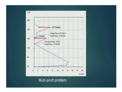
Now this is a G C C of a process, which has got multiple pinch this one is the utility pinch the heat flow is 0, here this is the process pinch the heat flow is 0. So, it has got multiple pinches you can have more than one utility pinches also, if we face such a problem then will try to avoid it for integration.
