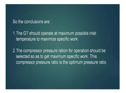
So the conclusions are the GT should operate at maximum possible inlet temperature to maximize specific work. This is one conclusion the second the compressor pressure ratio for
