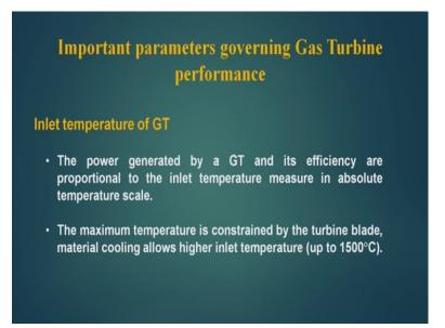
Now if you see the inlet temperature of G, the power generated by a gas turbine and its efficiency are proportional to the inlet temperature measured in absolute temperature scale. The second thing is the maximum temperature is constrained by the turbine blade, so see turbine blade decides that what should be the temperature of the gas which is entering into the turbine. If material cooling is allowed then higher inlet temperature up to 1500 can be reached.
