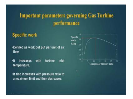
Specific work - it is defined as work out put per unit of air flow it increases with turbine inlet temperature. It also increases with pressure ratio to a maximum limit and then decreases and then this is the same of the curve.
