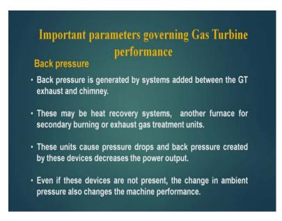
Backpressure - the backpressure is generated by systems added between the gas turbine exhaust and chimney like a recuperator. This may be heat recovery systems, another furnace for secondary burning or exhaust gas treatment units. These units cause pressure drop and back pressure created by these devices decreases the power output. Even if these devices are not present, the change in ambient pressure also changes the machine performance.
