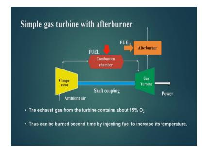
Now if you see analyze the exhaust gas then we find that the the exhaust gas from the turbine contains about 15 percent oxygen. So we can only add fuel to it, and we can re-burn it, so that the temperature of the exhaust gas can increase.
