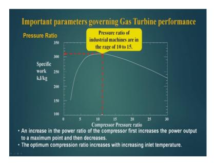
Second thing is pressure ratio. Now if you see the compressor pressure ratio here, this specific work, this is the work done per kg of the air takes such a unimodel shape. An increase in power
