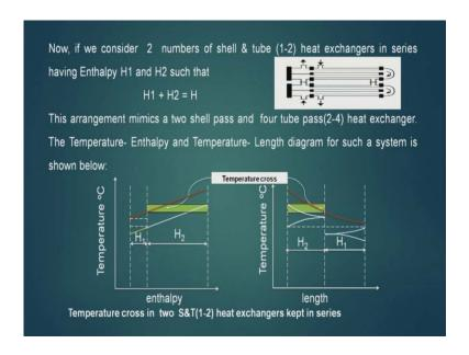
So, my aim will be to improve the F T factor. So, the improvement can be done by joining two one to seven tube heat exchangers in series. So, now, we consider two numbers of shell and tube heat exchangers in series having enthalpy H 1 and H 2 such that H 1 plus H 2 is H and this is H is our demanded H P enthalpy; that means, the load for heat exchangers. This arrangement mimics a two shell pass and four tube pass heat exchangers which is called 2-4 heat exchanger.
