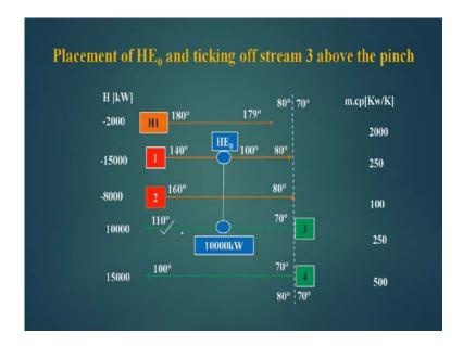
And place between 1 and the 3 streams and the heat carrying capacity of this stream is 10000, so it can be tick off this stream, because why the placing matches will be using the tick off rule to decrease the number of heat exchangers. So, we have use the tick off rule and they found that, this match is as for the rules and regulations of the pinch. Now, if I do this these stream temperature is dropped up to 100 degree centigrade, when I pass on 10000 Kilowatt from this stream.
