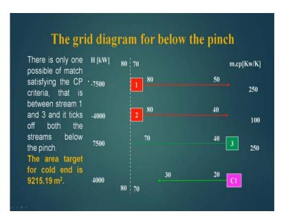
Now, the area target for the cold end design is 9215.19 meter square, now if we see this there is only one possible match satisfying the C P criteria, and that is between stream 1 and 3. So, stream 1 and 3 can be matched, because this is 250 and 250.
