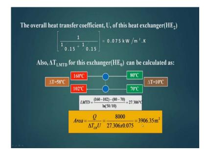
So, we calculate the heat transfer area requirement for this, so it is heating up to 102 degree centigrade, so here this is 58 delta T and here this is 10, so LMTD is 27.306 degree centigrade area is given by this. So, 8000 divided by 27.306 into 0.075, so area comes out to be 3906.35 meter square, so now, we go for the calculation for the second match also.
