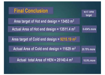
Now, the complete conclusions or final conclusions are this, area target of hot end design was 13453 meter square, actual area of hot end design was on 13511.4 meter square, so it was quite close to the targeted area of hot end. And the error was 0.0434 percent, so the area was 0.434 percent more, the area which we all Z through design, but the situation is not that good for the cold end design, the area target of the cold end design was 9215.19 meter square.
