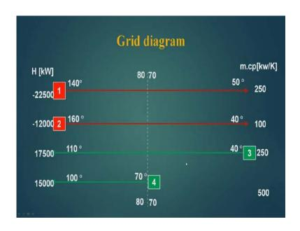
So, this is a stream diagram of the problem, the pinch is at 80 degree centigrade and 70 degree centigrade that means, hot pinch at 80 degree centigrade and cold pinch is 70 degree centigrade. So, with this free diagram, now we will divide this into two parts, the upper pinch area which is shown by this, this part is upper pinch and this part is lower pinch or we call this part is hot end and this part is cold end.
