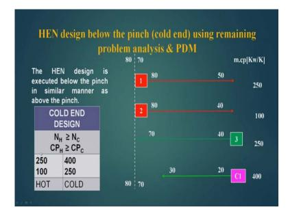
And my rule tells that my C P H should be greater or equal to C P C, so this is equal to 250 is equal to 250, then only this match can take place, this match cannot take place because 100 is less than 250. So, I have only one possibility of matching, so there is no alternative available and hence, I have to go for that matching and then, this stream will be left out which will be cooled down by the coolant that is cold utility C 1.
