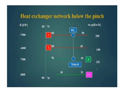
So, if I put that match which is the only available match, this available match is 7500 Kilowatt and this is going to tick off this both streams, because this is 7500 and this is 7500.
