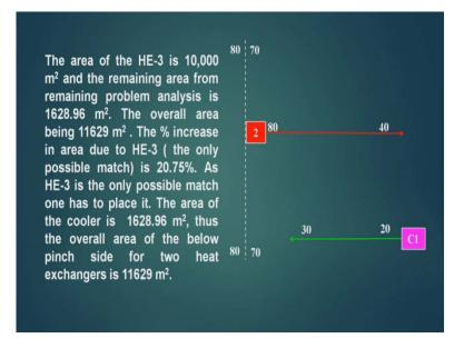
Now, the remaining problem is this, now when I find out the area of the heat exchanger number 3 by the same type of calculations, which has been shown earlier it comes out to be 10000 meter square. And the remaining area for the remaining problem analysis is 1628.96, so area computed for this remaining problem is 1628.96, so the overall area is 11629 meter square.
