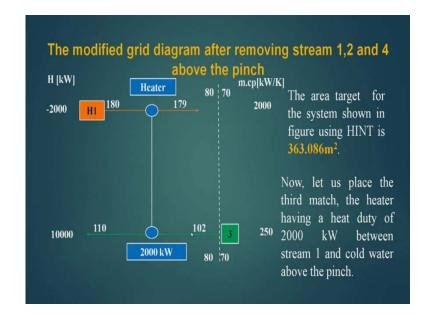
Now, let us place the third match, the heater having a heat duty of 2000 Kilowatt between stream 1 and the cold stream above the pinch, so you put a match here, this is a heater and this capacity is 2000 Kilowatt. Now, what we will see from here that in this design we have able to match the hot utility requirement, which was 2000 Kilowatt we are able to match this is, but the area requirement as been increased by 0.4 percent.
