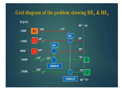
So, the first match we already accepted, because it is not taxing the total heat area of the heat exchanger network match on the 0.4 percentage or so, now we put the second match. Now, the second match will not tick off this, second match will tick off this and there will be it will heat the stream number 3 from 70 degree centigrade to 102 degree centigrade. And from 102 degree centigrade to 110 degree centigrade it will be heated by H 1 and then only it will ticked off.
