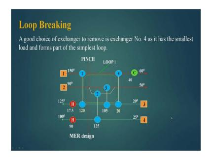
So, we take the first part of it. Now suppose we want to break the loop, a good choice of the heat exchanger to remove the heat exchanger 4 as it has the smallest load and forms the part of the simplest loop. Now if you see this, this heat exchanger number 4 has got the smallest capacity 20, and hence this is the ideal heat exchanger to be removed.
