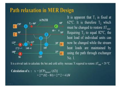
So, let us see this 4 goes there. So, now the capacity of this heater, cooler and this heat exchanger are changed.
