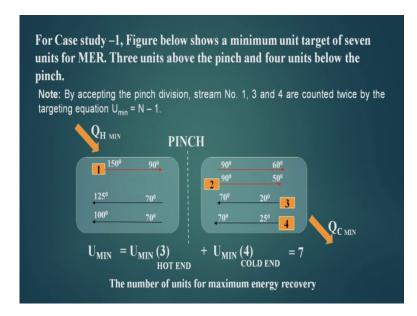
Now for the case study one figure below shows a minimum target of seven units of MER. Three unit above pinch and four unit below the pinch. Now if I apply the units target here, so there are four; that means, three process stream and one utility stream that makes it 4 minus 1, so there are three number of heat exchangers will be placed here including the heater. If I put the target units target here, so there are four process stream
