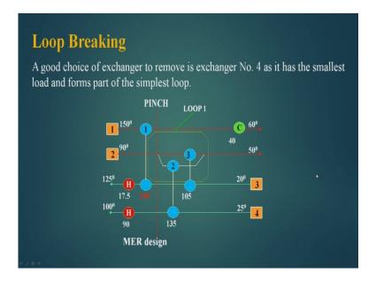
So, if I remove this heat exchanger then its capacity has to be added to this. So, this becomes 140, after transferring.
