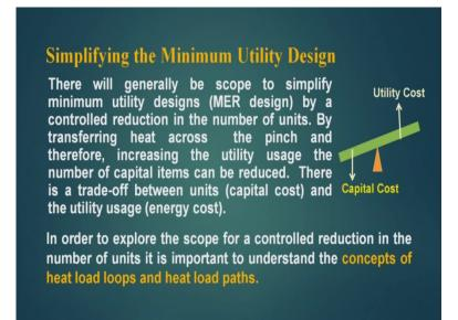
Now let us see there will generally be scope to simplify minimum utility designs that is MER designs by a controlled reduction in the number of units. By transferring heat across the pinch and therefore, increasing the utility usage the number of capital items can be reduced. There is a trade-off between the unit capital cost and the utility usage energy cost; here if you are decreasing the capital cost, the utility cost increases. So, how to balance this is main job.
