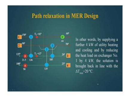
And then this temperature becomes 82 and this are changed capacity. So, in other words, by supplying a further a 4 kilowatt of utility heating and cooling and by reducing the heat load on exchanger number one by 4 kilowatt, this solution is brought back in line with the delta T minimum 20 degree centigrade.
