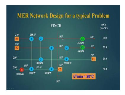
So, we have see that we are able to decrease a heat exchanger by breaking one loop. Similarly, we can also break the second loop and decrease the heat exchanger cost or the number of heat exchanger by one, so that we reach the minimum heat exchanger level that is seven in non-MER design. In the last design, the heat is passed through the pinch and thus after the loop breaking, the design coverts to the non-MER design.
