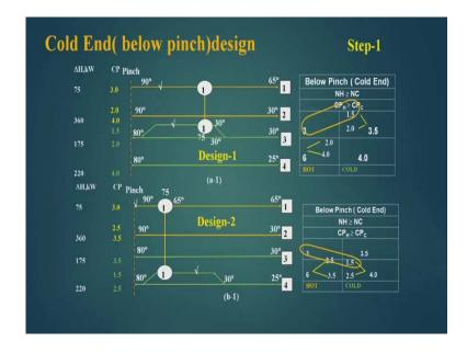
Now, we will go for the cold end design. Now, in cold end design, if you see the rules are then reversed here, the number of hot streams should be more or equal to number of cold streams. C P H should be greater than or equal to C P C. These are the 2 rules, which have to be obeyed for the cold end design. If 1 role is violated, then we have to split this stream to remove the violation or we can restrict to cyclic matching.
