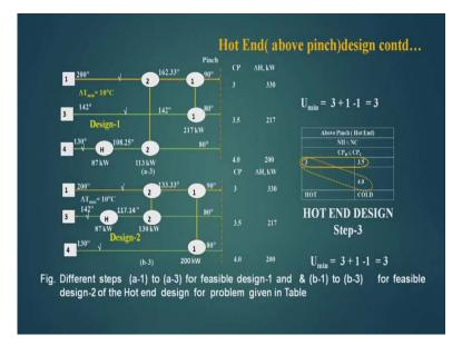
Now, let us see the second step. Now, it is step 2. Here, we have already put 1 on heat exchanger. Now, we will put second heat exchanger. Now, second heat exchanger can be put from hot stream to the fourth number cold stream and the hot stream to the third number hot stream to the third number cold stream. This is perfectly permissible because C P H should be less than or equal to C P C.
