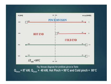
Now, this is the stream diagram or the grid diagram for the problem. The pinch temperature is hot pinch temperature is 90 degree centigrade and the cold pinch temperature is 80 degree centigrade. Q H minimum is 87 kilo watt. Q C minimum is 40 kilo watt. This has been observed. This result has been observed from PTA. That means we have already done the utility targeting and from the utility targeting, this result has come that is Q H minimum is 87 kilo watt. Q C minimum is 40 kilo watt.
