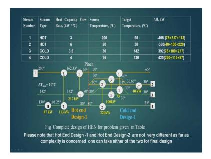
So, this is my complete design when I am mixing designs hot end design one and cold end design one. So, please note that hot end design one and hot end design two are not very different as far as complexity is concerned. One can take either of the 2 for the final design.
