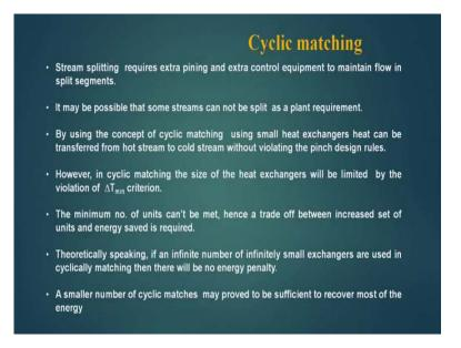
Stream splitting requires extra piping and extra control equipment to maintain flow in split segments. It may be possible that some streams cannot be split as a plant requirement, by using the concept of cyclic matching using small heat exchangers heat can be transferred from hot streams to cold stream without violating the pinch design rules.
