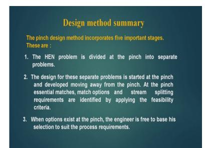
So, let us have the summary of the design methodology. The pinch design method incorporates 5 important stages these are, the hen problem is divided at the pinch into separate problems. So, the total hen problem is divided into the pinch by upper half reason, lower half, upper half is hot end and lower half is cold end. So, the pinch design methodology divides the hen problem into two distinct or separate problems, which are thermally in equilibrium or thermally sufficient.
