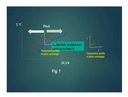
Now, this is the suppose this is the this is a composite curve, here this is expanding that means this distance is minimum. Here it is more here it is more and more. Now, here if I am tracing a heat exchanger here, the temperature profiles of the heat exchangers length is this. If this matches with here then the design will give minimum area. So, it matches here now that can be a case where they are not matching say this is a case where it is not matching.
