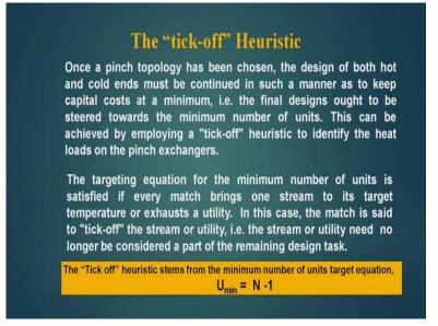
Once a pinch topology has been chosen, the design of both hot and cold ends must be continued in such a manner as to keep capital costs at a minimum. We have already told that when we are designing a heat exchanger network, then the designs will take place in such a way that the cost is minimum, the final design ought to be steered towards the minimum number of units.
