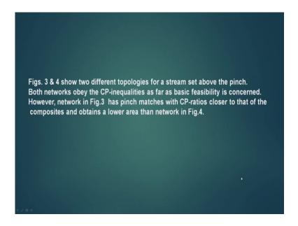
So, this rule also tells me that how to put the different matches based on CP ratios. So, concluding figure 3 and 4 shows different topologies, for a stream set above the pinch. Both networks obey the CP inequalities as far as basic feasibility is concerned. However network in figure 3 has pinch matches with CP ratios closer to that of the composites and obtains a lower area than network 4. So, our CP rule is over.
