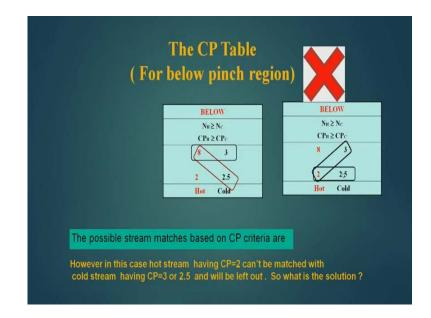
The possible matches are here CP H Should be greater than CP C. So, I can do this matching because 8 is more than 3 or I can go for 8 is more than 2.5. So, I can take this match as well, if I want to do the matching like this 2 to 3 or 2 to 2.5, this is not permissible because this violates this criteria CP H greater or equal to CP C. Here CP H
