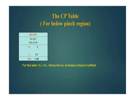
In this condition N H is equal to N C because there are two hot streams and two cold streams so this criteria is fulfilled.
