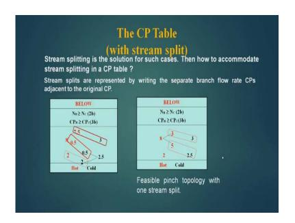
Then the question is how to accommodate the stream splitting in the CP table. Stream splits are represented by writing the separate branch flow rate CPs adjacent to the original CP. Now, if we want to split the stream which has got a CP value of 8 we will write down the adjacent CPs 7.5 and 0.5 here, with a line like this. So, it is all that the 8 is spitted into 2 streams out of which 1 stream has a CP of 7.5 and the other stream has got a CP of 0.5.
