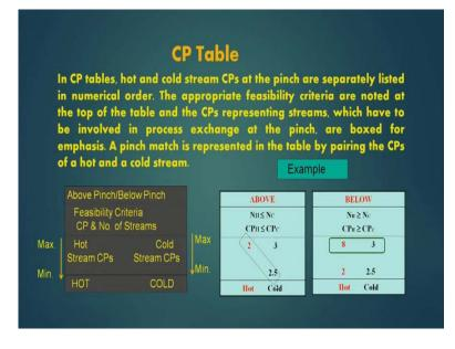
Now, in this lecture the rest will be covered. To start with it will start the CP table, in CP tables hot and cold streams CPs at the pinch are separately listed in numerical order. The appropriate feasibility criteria are noted at the top of the table. The CPs representing streams, which have to be involved in process exchange at the pinch are boxed for emphasis. A pinch match is represented in the table by pairing the CPs of a hot and a cold stream.
