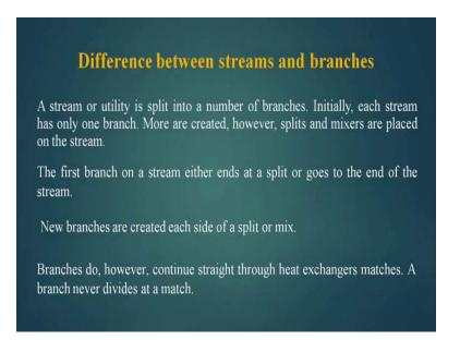
A stream or utility is split into a number of branches, initially each stream has only one branch, more are created. However, splits and mixers are placed on the streams, the first branch on a stream either ends at a split or goes to the end of the stream, this will see when, is split a stream. New branches are created each side of a split or mix, branches do however continue straight through, heat exchangers matches, a branch never divides at a match.
