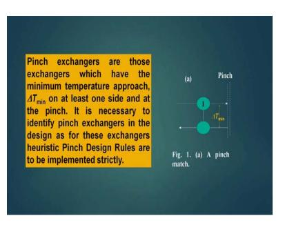
Pinch exchangers are those exchangers, which have the minimum temperature approach delta t minimum on at least one side and at the pinch. It is necessary to identify pinch exchangers, in the design. As for these exchangers heuristic pinch design rules are to be implemented strictly. Now, if you see this figure this is heat exchanger 1, if you see this pinch side of it, these are the two streams, which are touching pinch.
