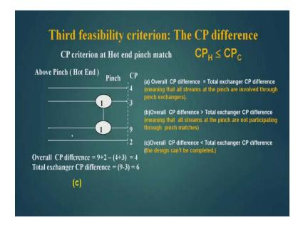
Now in this case, overall CP difference is more than the total exchangers CP difference. Now let us see a part c of this now, there are 2 hot streams and 2 cold streams and there is only 1 match so, the overall CP differences is 9 plus 2 minus 4 plus 3 is 4 and total exchanger CP difference is 9 minus 3 is 6. So, here the overall CP difference is less than is total exchanger CP difference so, we will saw there are three different result a, b and c.
