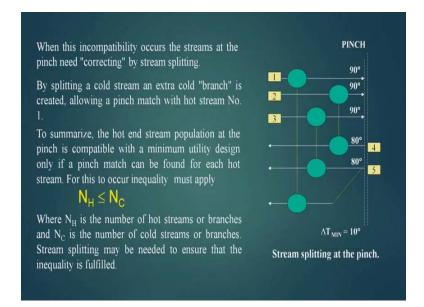
Now by splitting a cold stream an extra cold branch is created, allowing a pinch match to the hot steam. So, the solution is splitting a steam at the pinch so, if I split this original team into two parts, one part this, another part this then, the temperature of this part will increase 80 plus delta t. But the temperature this part remains at 80 degree centigrade and hence, I can put a match from 1 to the split stream of number 5.
