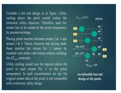
Now, suppose we put to matches here between hot stream 2 and cold streams number 4, hot steam 3 and cold stream number 5. If suppose d Q amount of heat is pass from 2 to 4, this temperature 80 degree will increase now. Similarly, this 80 degree temperature will increase by passing of d Q amount of it. Now, if it is so, then there will be a problem in matching, which is low that the pinch divides the problem at two parts, upper pinch and lower pinch or hot end and cold end.
