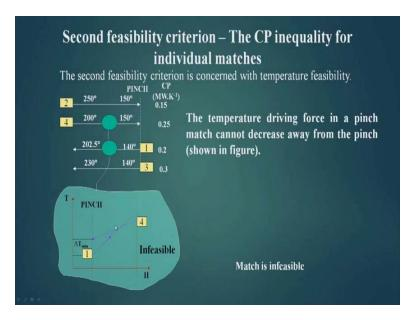
Now, the second feasibility criteria, the CP inequality for individual matches, now the second criteria is what, it tells about the matches that means, the stream should be matches with streams, which hot streams should be match with cold streams. The second feasibility criteria is concerned with temperature feasibility, this is the small problem is seen, there are 2 hot streams, 2 cold streams.
