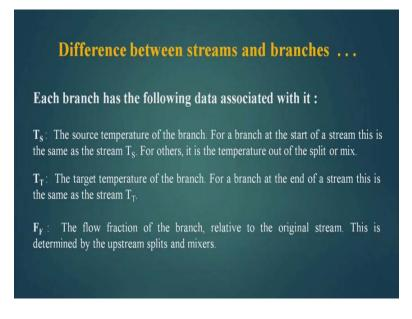
What are the difference between streams and branches, each branch has the following dada associated with it. T s that is, supply temperature or the source temperature, the source temperature of the branch, for a branch at the start of a stream, this is the same as the stream T s. For others it is the temperature, out of the split or mix similarly, T t which is the target temperature of the branch, for a branch at the end of a stream, this is the same as the stream T t.
