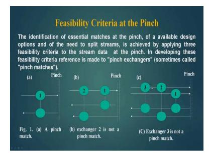
The identification of essential matches at the pinch of a available design options and of the need to split stream is achieved by applying, three feasibility criteria to the stream data, at the pinch. At the pinch is very important for us and there are a lot of restrictions at pinch so, we will use three feasibility criteria for the pinch matches. Now, here let us see again what are the pinch matches this is obviously a pinch match, this is a pinch match, but this is not a pinch match.
