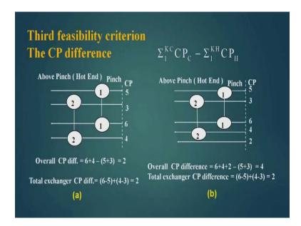
So, we take the hot pinch area now, the overall CP difference in 6 plus 4, this is the CP of two cold streams, 6 plus 4 minus two hot streams, 5 and 3, 5 plus 3. So, this overall CP difference is 2 so, I am using this equation and individual CP differences that is total exchanger CP difference if you see then this exchanger matching with this so, this is 5 minus 5 and for this is exchanger this is 4 minus 3.
