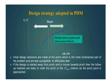
The design should start from here at pinch and this, then should go away from the pinch, for this side also and for this side also. So, this is above pinch area and this is the below pinch area. So, for above pinch area we know that, the pinch, divide the problem into two parts, above pinch area and below pinch area.
