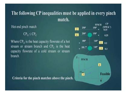
Now, here we see that when we will put match between 4 and 3, this diversions take place and now, the delta t available here, is very less that means, larger than 10 degree centigrade, which is available here at the pinch. So, this is diverging that means, delta t is available here, here or here is more than this. So, this is a proper matching, this matching is a proper matching, but what made this, if we analyse this has something to do with this CP value.
