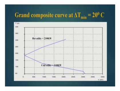
Now, if I plot it for delta T minimum equal to 20 degree, I clearly see that grand composite curve is changing. Here, the hot utility requirement is 2100 kilowatt, and cold utility requirement is 3100 kilowatt. I can show you the earlier one for a comparison, this is for delta T minimum 10 degree centigrade, and this is for the delta T minimum 20 degree centigrade.
