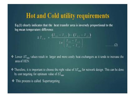
The log mean temperature difference can be computed using equation 2, which is also a well-known equation. So, I do not have to discuss it more. The lower delta T values result in larger and more costly heat exchangers as it tends to increase the area of heat exchangers. So, when I decreased the delta T minimum, the fixed cost of the heat
