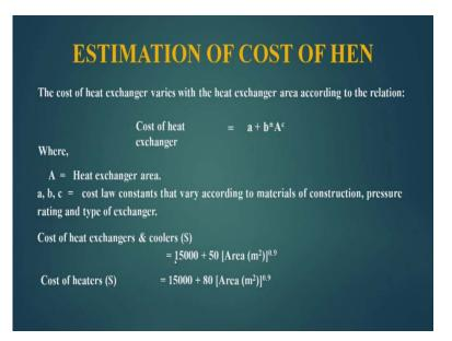
The cost of the exchanger varies with the heat exchanger area according to the relationship given below. Here we are using a plus b A to the power c. Where, a is the area of heat exchanger network, the cost of the heat exchangers and coolers are given like this. So, these are the cost formula, and here this is 15000 plus 50 area to the power of 0.9; and for the heaters, this is 15000 plus 80 area to the power 0.9, and this is for heat exchangers and coolers as well.
