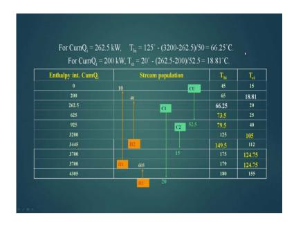
We are computing the unknown temperatures. This shows an example how to compute the temperature. So, this unknown temperature was computed using this equation. Similarly, we will fill it up T ci is equal to this known temperature minus this enthalpy values, and then we have also use the summation of C p
