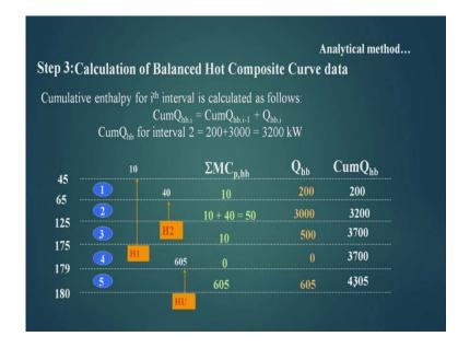
Now, cumulative heat available in these intervals is necessary to plot the hot balanced hot composite curve. So, we find out cumulative and this is the value is 200. For this temperature level, it is 3000 for plus 200 that is 3200, so this is 3200. And for this, it will be this value plus this value plus this value and so on so forth.
