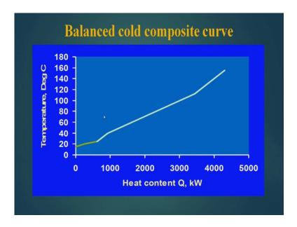
Then we have to put these two curves in one plot, so that the delta T minimum is 20 degrees centigrade.
