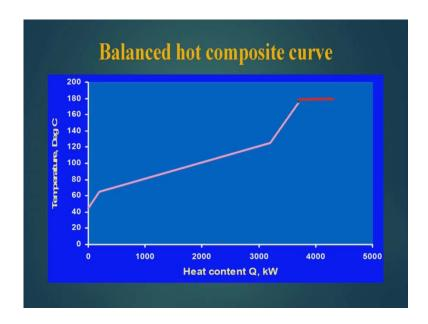
Now, based on that cumulative value and the temperature levels, we can plot the balanced hot composite curve. Now our balanced hot composite curve is ready. So, the next step is to find out data for plotting the balanced cold composite curve.
