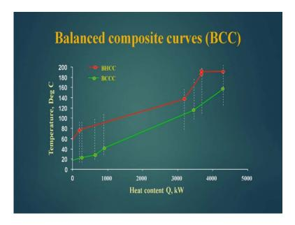
Now this point is you see that in the balanced hot composite curve or the balanced cold composite curve, where the line is changing slope that point is known. Because this is the point, where either the inlet temperature or the outlet temperature of the stream individual stream exists, so that is why these temperatures are known where the slope is changing. So, this temperature is
