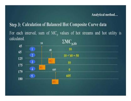
Now, we will compute the M C p values for hot streams at different temperature intervals. This is 10, because in these temperature intervals 65 to 45, there is only one hot stream present, and its M C p value is 10. But in this temperature interval 125 to 65, two hot streams are available whose combined M C p value is 10 plus 40 is equal to 50 and so on so forth. We can fill up this column.
