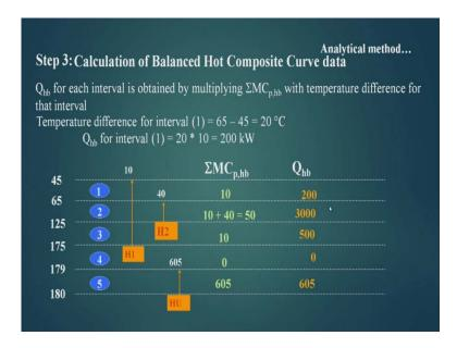
Now, we can calculate Q hb - that means what is the heat available in this temperature intervals, because we are integrating based on temperature intervals.
