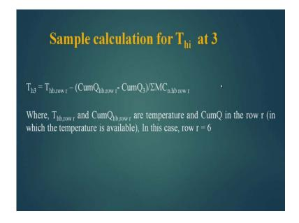
So, these are the equations through which we do this is basically a linear interpolation equation, and we have discuss this in area targeting. So, I am quickly skip this.
