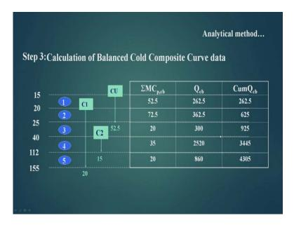
So, for the balanced cold composite curve, in the similar manner, we have computed the M C p of cold composite curve then Q cb then cumulative Q cb. Once these data is known to us, we can plot the balanced cold composite curve.
