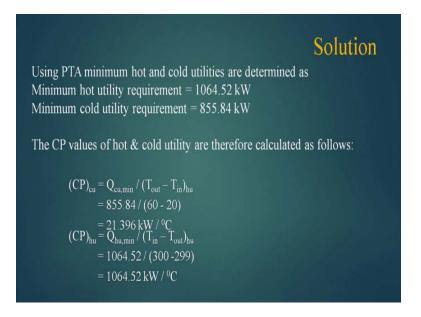
Now once the stream table is available, we can go for problem table algorithm PTA to find out, minimum hot and cold utilities. If we do this, we find that the minimum hot utility requirement is 1064.52 kilowatt, minimum cold utility requirement is 855.84 kilo watt. Now based on these values of hot and cold utilities, we will try to find out what
