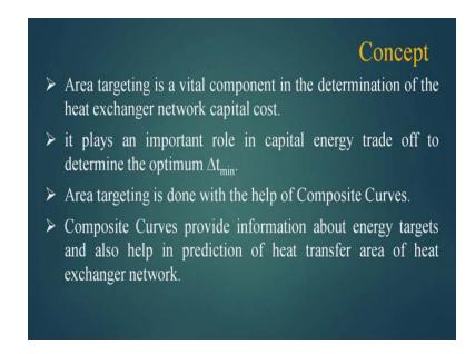
Area targeting is a vital component, in the determination of the heat exchanger network capital cost. It plays an important role in capital energy trade off, to determine the optimum delta t also. Basically, when we design a HEN using the pinch analysis for a given problem then, many heat exchanger networks can be created based on the value of delta t minimum. Then, an optimum delta t minimum is selected which keeps the tack of the HEN as minimum.
