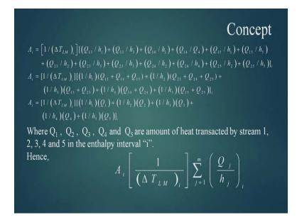
So, 1 by delta T LMi will be equal to Q 13 by h 1 plus Q 13 by h 3 plus Q 14 by h 1 plus Q 14 by h 4, Q 14 by h 4. Similarly, I can express this, then finally, I can find out by solving these equations, that the total heat transfer area of the ith interval will be given by 1 by delta T LMi summation j 1 to m Qj by h j of i.
