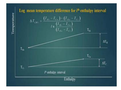
So, this shows how the delta T LM of the ith interval, enthalpy interval and be computed. So, this is delta T Hi minus T CO minus T HO minus T CI divided by this l n T Hi minus T CO, T HO minus T CI.
