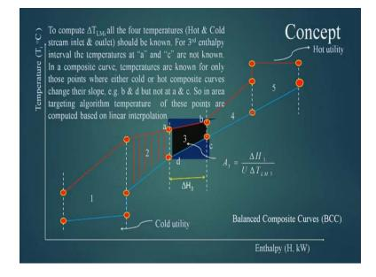
Further, if you see here, then you find that, there are few points which are not available. Like, if you see this number 3, that is third enthalpy interval, the temperature at a and temperature at c is known, temperature at a and temperature at c are not known in the composite curve.
