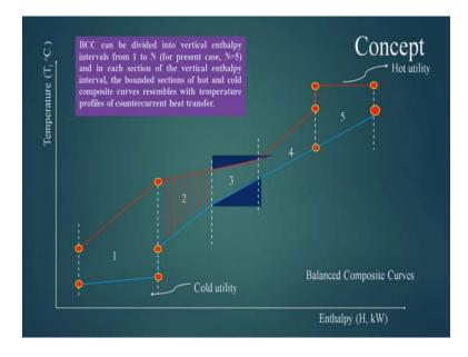
Now the figure shows a composite or a balanced composite curve, the upper one shows a balanced hot composite curve where, this part of the hot composite curve shows the hot utility. And this shows a balanced cold composite curve, where this part of the curve shows the cold utility. The balanced composite curve which is drawn between axes temperature and delta h, which is enthalpy, can be divided into vertical enthalpy intervals from 1 to n.
