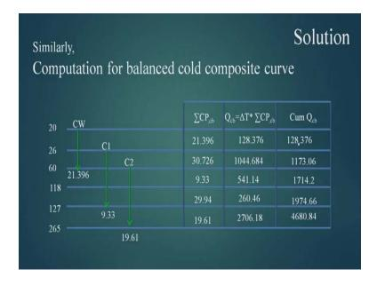
Now, we will see how to compute the data for balanced cold composite curve, for balanced cold composite curve, we will select from the stream table, the data for cold streams, that is C1 and C2 and cold utility. The temperature levels are written here as from 20, 26, 60, 118, 127 and 265 in the increasing order, the cold utility CW goes from 20 degree centigrade to 60 degree centigrade, to its CP, capital CP is 21.396.
