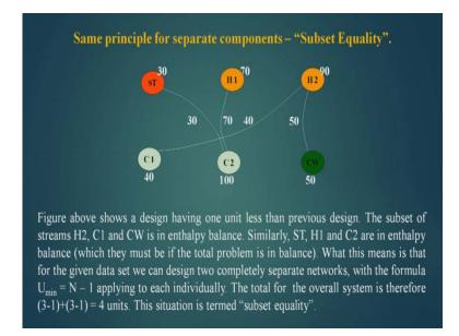
Now, the same can be done in this way - that means, H 2 gives 50 units of heat to cold water, and remaining 40 of units of heat is passed to C 1 then H 1 gives 70 units of heat to C 2 and remaining 30 to passed on by the steam to C 2. If I arrange this way, the heat exchangers I find that I am using one less heat exchangers that is 5 minus 1 equal to 4, and with four heat exchangers I am able to solve the problem. A special case we see that
