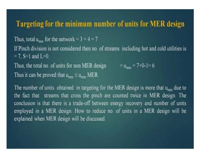
So, what we conclude out of this. If you do the targeting for the minimum number of units for the MER design, and what we find that U minimum for the network is 3 plus 4 is equal to 7 units. If pinch division is not considered then number of streams including
