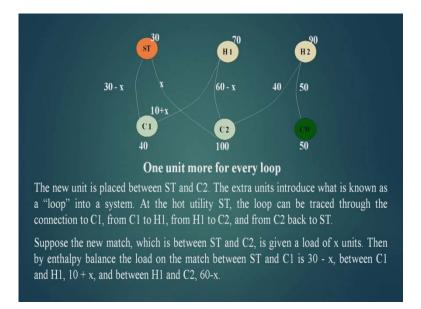
Now we see a second case, here I put a extra line between steam to C 2 which transfers x amount of heat. If it transfers x amount of heat to C 2, then 30 minus x amount of heat will be transfer to C 1, and 10 plus x amount of heat from H 1 will be transfer to C 1, and when we add 30 minus x plus 10 plus x it is 40, so it is C 1 is satisfied. Similarly 60 minus x will be transfer to C 2, and 40 units of heat come from H 2 to C 2, and 50 units
