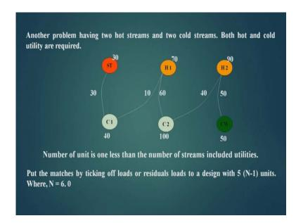
Now, let us see a problem with 2 hot streams, two cold streams a hot utility and a cold utility. Hot utility is give by ST, which is a steam; and cold utility CW - cold water. And hot streams are H 1, H 2; cold streams C 1 and C 2. The steam which is given by ST as
