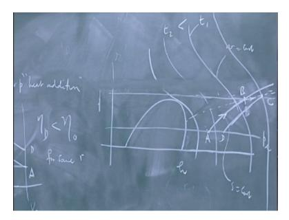
The diesel cycles are actually similar except that you have two parameters for control you have a vs and vc again it is a same contraction you have the exhauster can the inlet stroke what you have is a compression adiabatic compression and this stage the fuel is now added by injection and you cut off the fuel injection at some point then it goes like this so here it is constant pressure heat addition.
