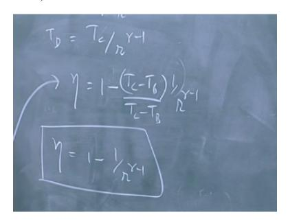
So your r is actually vs + vc this is stroke volume this is clearance volume if you want I will call this vcl to make it clear okay we have another vc by v clearance, clearance volume is the date volume if you like when the piston is at the top.
