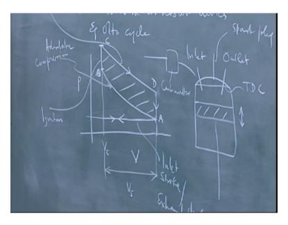
The quantity of interest is how much heat do you add here we write this in terms of q in actual fact it is a reaction occurring where as I told you internal energy as a product is less than the internal energy of reactance and therefore you get net heat added to the system but we calculated in terms of heat added and work done the heat added divided by the a calorific value of the fuel will give you the amount of fuel consumed.
