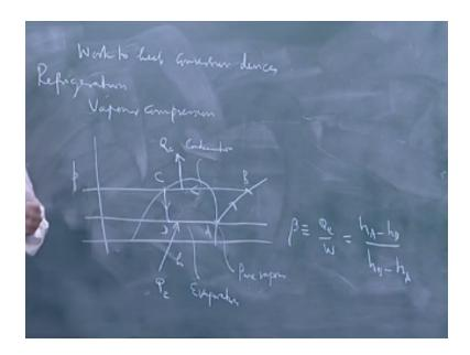
Because this is called vapor compression refrigeration which is what you would have done on the ph diagram and then I want o discuss later absorption refrigeration which is used in large scale this is work to heat conversion devices, here you are talking of two phases what you do is take let us say pure vapor could be free on now you have non florohydrocarbons for this thing but you have pure vapor which you compress a long an adiabatic.
