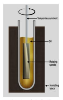
Unlike here it is flowing through gravity. In this direction g was acting. g was acting. Unlike here is the rotation. It is horizontally placed. And rather than function of the fluids internal shear stress or rotational visco I mean the rotational viscometer calculates the absolute viscosity.
