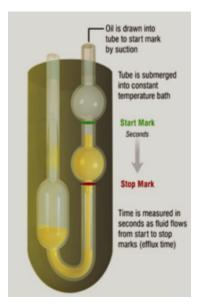
So combining all this there are three ways the viscometers are designed. One is capillary or glass viscometer, rotational viscometer and falling ball or falling piston viscometer. These are the three which encompasses the three basic principles, basic methods that is in the green color suit in the left side of it. But these are the measurement techniques. By the way, before going to the viscometer and rheometer, see it grossly comes under the head of rheometry basically.
