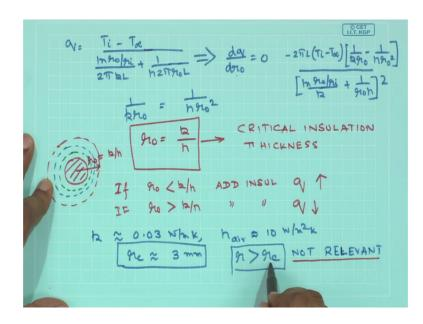
So, starting with this q which is I will write it again T i minus T infinity by ln r naught by ri twice pi k L plus 1 by h 2 pi r naught L I am going to differentiate this and set this to be equal to 0. So, I am trying to find out is there a radius r 0 where r 0 is the insulation thickness which would maximize the flow of heat which is denoted by q.
