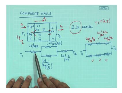
But before I conclude this part of the class let us just briefly for 2 minutes; we look at composite walls which are slightly different. Let us say you have a system in which up to this point is mid is made of some material and from this point onwards it is of another material, but in between you have 2 different materials.
