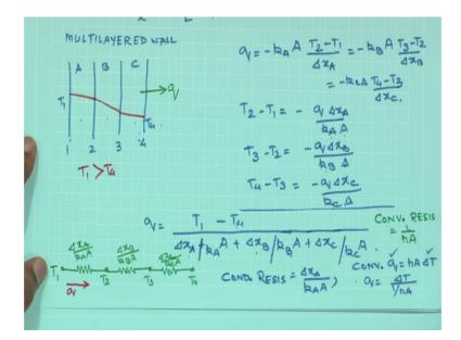
So, we will go back to the we are we are going to do something else with this equation, which simply tells me that q double prime x q double prime x is equal to k by L T 1 minus T 2 ok.
