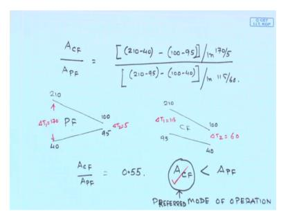
So, therefore, to write this the area required for counter flow divided by the area required for parallel flow would simply be the log mean temperature difference for the case of parallel flow which is, this is the delta T 2 minus delta T 1 divided by ln 170 by 50. And, for the case of count for the case of counter flow the l m T d for the counter flow would be 210 minus 95 minus of 100 minus 40, this divided by ln 115 by 60.
