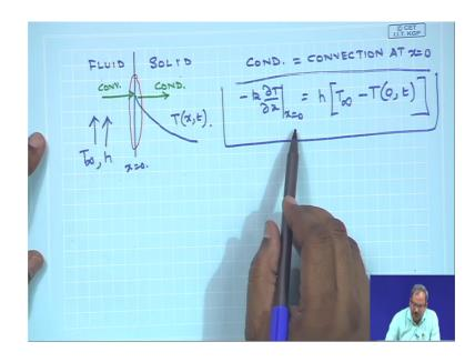
So, what you have then, I will I will I will draw it once again. This left he solid side, this is the fluids fluid, the fluid is moving with a velocity with some velocity having a temperature T infinity and with a convection heat transfer coefficient as h, and let us say that the fluid temperature is more than that of the solid. So, this is how the temperature inside the solid would change with time.
