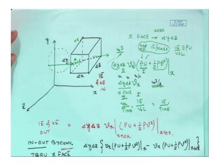
So, after that what I have, what I have done is I have defined the volume element in here, as this is the volume element and I have identified what are the terms for convection.
