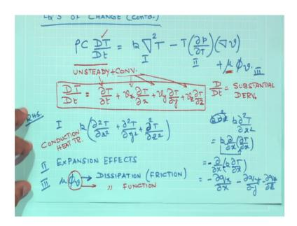
So, when I combine all these terms together and divide the, divide both sides by del x del y del z and then, take the limit when all of them approach to 0. What I get is a reduced form of the, reduced form of the equation and I am going to write the final form of the equation as rho C D temperature by D time is equal to k del square T, divergence of T minus T of del P del T times velocity, this is velocity plus mu phi v.
