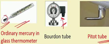
Ordinary mercury in glass thermometer      Bourdon tube      Pitot tube
