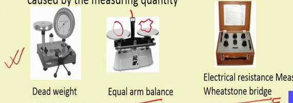
Dead weight pressure gauge      Equal arm balance      Electrical resistance Measurement by Wheatstone bridge
