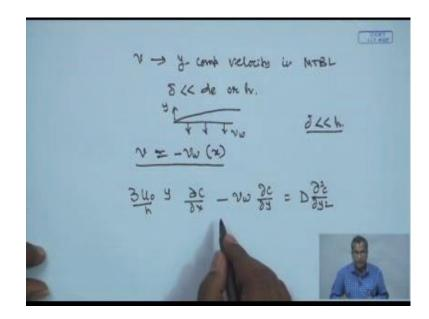
V is the y component velocity in mass transfer boundary layer and we assumed that since we have already founded that delta is much-much less than effective diameter or channel half height. So, therefore, the thickness of mass transfer boundary layer is probably less than 1 percent of the channel dimension and it is really very very small.
