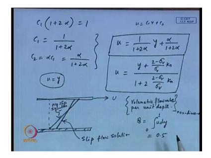
And so what you end up with in that case is I can write hereas c 1 into 1 plus 2 alpha that is equal to 1, c 1 you bring all the c 1 to the left hand side, and so you get c 1 into 1 plus 2 alpha is equal to 1 oryou get c 1 is equal to 1 by 1 plus 2 alpha c 2 we had alpha c 1 that means, equal to alpha by 1 plus 2 alpha. So, earlier, we had what, we had c 2 is equal to 0 and c 1 is equal to, we had capital u divided by h.
