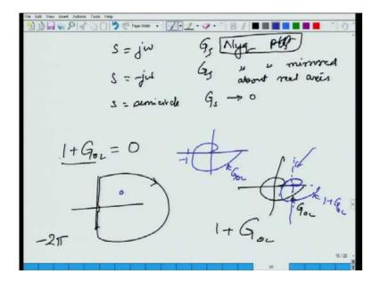
On s equal to j omega, you get Nyquist plot on s equal to G, s is essentially the Nyquist plot on s equal to minus j omega G, s is Nyquist plot mirrored about real axis, and s equal to semicircle. Usually what will happen is G s maps to 0. So, you can see that for more realistic system, just the Nyquist plot contains all the information and now getting back to, what I am actually looking for is the encirclements, the right half plane pole; the right half planes roots of this equation yeah.
