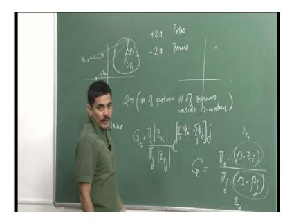
So, this is the s plane, and I have s moving on a contour, I have a got a pole inside, and I have got 0 here, and may be may be a pole here. So, this one is p 1, this was p 2, and this was z 1, and what I was saying was, this is s minus z 1, then this is si 1, this is s minus p 1, and this is phi 1 and this is s minus p 2, and this guy is phi 2 and corresponding to this
