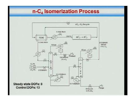
Now here is the process you have a C 4 feed stream, there is the C 4 feed stream, and this feed stream is containing C 3 propane, i C 4 and n C 4 isobutene and normal butane, and i C 5 iso pentane. So, the feed is mostly normal butane, little bit of C 3 and little bit of C 5 impurities. Now this feed is sent to a d isobutanizer DIB, de isobutanizer column, it is a
