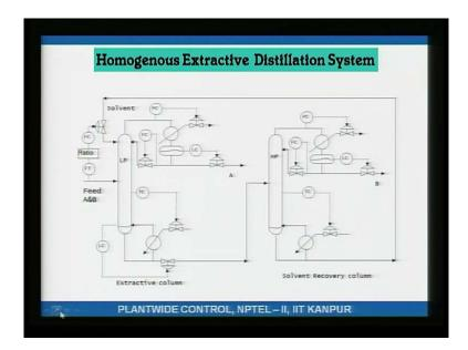
And that when the purity starts to decrease even though L by D is being increased you must become aware that the solvent to feed ratio needs to be increased in this control structure that is about it. So, we have talked about heterogeneous extractive distillation system. Next class, which will be the last class on distillation systems, we will look at some complex column configurations and their control and after that we will end, then will go onto control of reactors.
