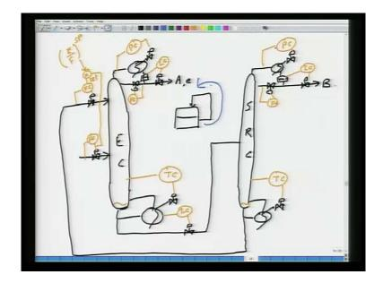
So, we are looking at the homogeneous extractive distillation sequence. The sequence looks like this I have got the extractive column which takes in the feed. And the solvent some place up there or the entrainer some place up there, because it is got a condenser reflux drum and reflux. The top stream is essentially, let us say pure A, and some amount of E bottoms is essentially B this is called the solvent recovery column.
