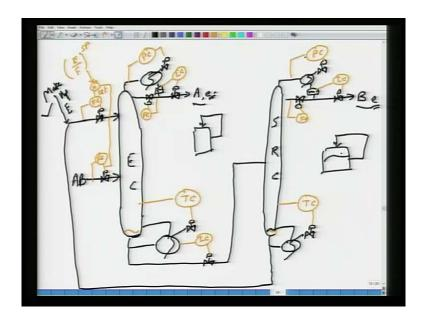
Similarly, if you look at this process like a tank, then I am putting in an A B feed I am taking out A I am taking out B, the entrainer is simply circulating round and round. So, that is like this recirculation stream
