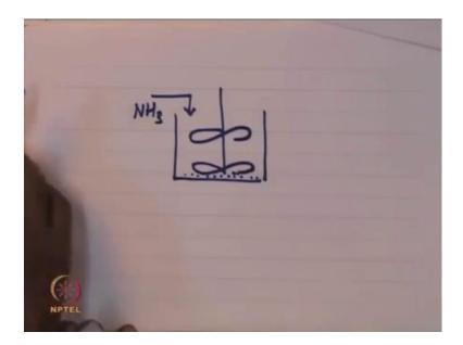
See in the industry, you also see this you have a batch equipment and very carefully designed stirrer in a this stirrer you know it is and then PH adjustment reactor is a batch reactor where you put ammonia add to adjust the PH. But here, what you have to do is that? You have to keep the agitation and then this enzyme at be sitting some like here and it is be done very carefully, most experience of process is that it is not easy to do it and therefore, people have thought of doing like this.
