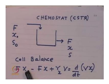
So, let me quickly explain to you what is the fundamental that you have to understand So, what is it that we have we have a chemo stat what is the chemo stat chemo stat is c s t r where feed comes in continuously feed goes out continuously, and because of the of the process that take place in this equipment. This S naught which is a pollution level comes down to S.
