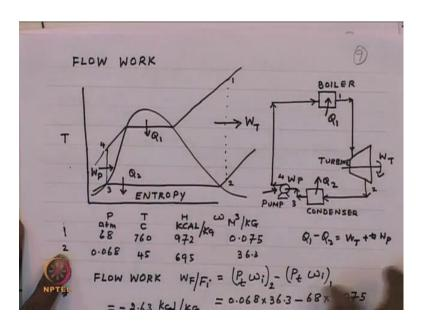
So, let us see what happens in a stream turbine? Stream turbine we have done in a way we have already calculated the stream turbine; we have calculated here. If we do this same calculation for this stream turbine is about the minus 0.2.63. So, we can calculate the flow work required for a stream turbine or for a sulfur dioxide.
