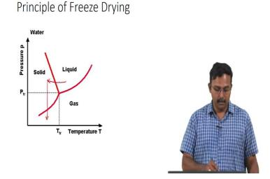
Let us look at the phase diagram for water. This is a simple phase diagram plot between pressure versus temperature for water. You have three phases, you have the solid phase, you have the liquid phase, and you have the gas phase.
