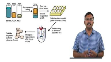
Let us first talk about the solvent casting and salt leaching method. So, this is an example of how you would use this method to prepare a scaffold. In the protocol given, you have three things; first is the solvent, which can dissolve the polymer and the salt which you are using for this method.
