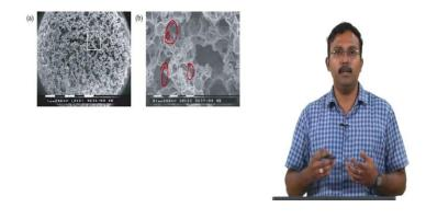
The scaffold which you have prepared using gas foaming and salt leaching method would look something like this. So, what you see here are pores that have good interconnectivity. Because the gas is pumped through the pores, you would have nice interconnectivity for the pores.
