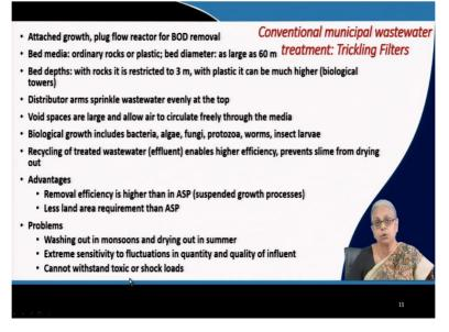
Just to give you an idea, there is a little bit information about trickling filters as well over here. So, we have attached growth process. Trickling filters are an attached growth process. They are generally run in plug-flow mode. But if you have a significant amount of recycling of the biomass; the greater the amount of recycling, the closer it begins to resemble a CSTR.
