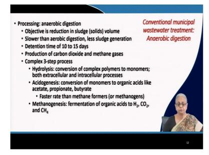
Then we come to the second microbial process or biological process and that is anaerobic digestion. Now, this process has been getting a lot of attention for 2 reasons. One, it has been used initially for wastewater treatment, but now it is also getting attention for its ability to be used for municipal solid waste treatment. So, the same thing applies to both types of wastes, and it is becoming more and more popular.
