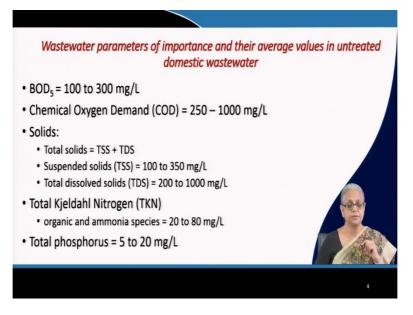
So, why are we using microbial processes or biological processes for treating wastewater? So, these wastewater parameters that are of importance in untreated domestic sewage or wastewater are basically shown over here in this slide. So, we have BOD<sub>5</sub>. Now, remember that is our standard method. So, the BOD values tend to range from 100 to 300 mg/L; COD ranges from 250 to 1000 mg/L.
