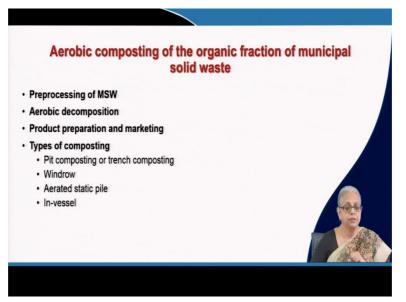
What is required in aerobic composting? So, composting is an aerobic biodegradation process. You need to segregate; the first most important thing is, you need to separate the organic fraction of municipal solid waste from the remaining part of the waste. Then, that organic material can be decomposed under aerobic conditions. So, the only thing you need to do for maintaining aerobic conditions is to provide some turning.
