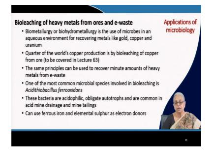
Then we come to the last application that I want to cover in this course, and that is bioleaching of heavy metals from ores and electronic waste. These processes are collectively called biometallurgy or biohydrometallurgy, for the simple reason that you cannot have biological processes without water. So, biometallurgy implies the presence of water, and therefore it is also called biohydrometallurgy.
