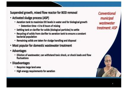
As I said, I will go through a little more detail about ASP or activated sludge process. So, we have a suspended growth process with a reactor that is a completely mixed flow reactor.
