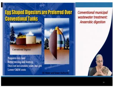
These are examples of different types of anaerobic digesters. Way back, 50, 60 years ago, people used to use digesters like these. These are what are called conventional digesters (image on the left). So, they were very large cylindrical tanks. They either had fixed covers or floating
