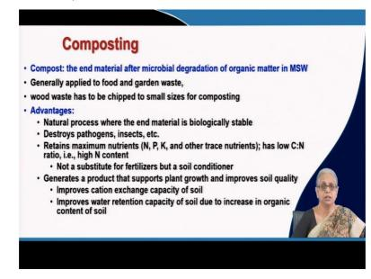
Here we come to another process and that is composting. Composting in India, we believe has been around for ages, literally. And what is composting? Composting is when you utilize waste organic material and convert it utilizing natural microbial degradation processes, and you get an end product which we call compost. Now, this compost is considered to be; many people consider it a substitute for fertilizer, but I would say that the best description of compost is that it is a soil conditioner.
