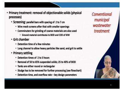
Then we come to primary treatment. Now, primary treatment of wastewater is based on physical processes only. So, I am just giving you a very quick overview of these processes, even though there is no microbiology, no application over here. So, primary treatment is the removal of objectionable solids, it is a physical process. I have already mentioned that parallel bars and wire mesh screens are used.
