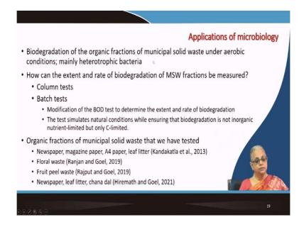
Let us now come to the second part. So, now we can take a look at another test. So, using the same principle as the BOD test, we have now come up with an aerobic biodegradation test to determine, or rather, let me put it another way; using the same principles that are part of the BOD test, we have taken the same ideas and transferred them to measuring the biodegradable fractions or the biodegradable potential for different organic fractions of municipal solid waste under aerobic conditions.
