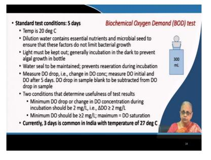
So, let us start with the biochemical oxygen demand test or BOD test. Now, this is a standard test that is used to determine the biodegradation potential of any wastewater. So, this has been in existence for probably 100 years or so (it was selected as a standard method in 1908). The standard test conditions are for 5 days. The temperature is standardized to 20°C. I think it started in the UK, and it has been more or less unchanged since then.
